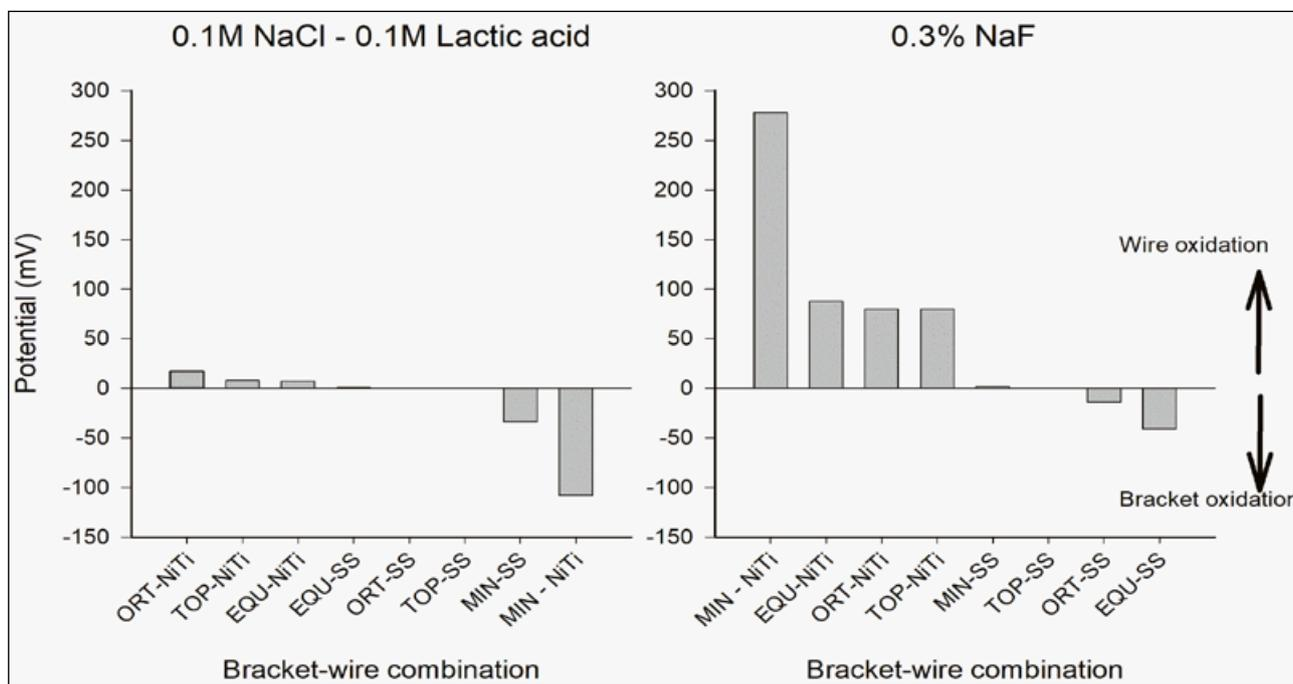
Figure 3. Mean potential differences for all bracket-wire combinations in descending order from left to right in both solutions tested. In all cases the standard deviations were found to be less than 23 mV and they are not presented for the sake of clarity. Positive mean values denote wire oxidation while negative depict bracket oxidation as shown by the arrows.
