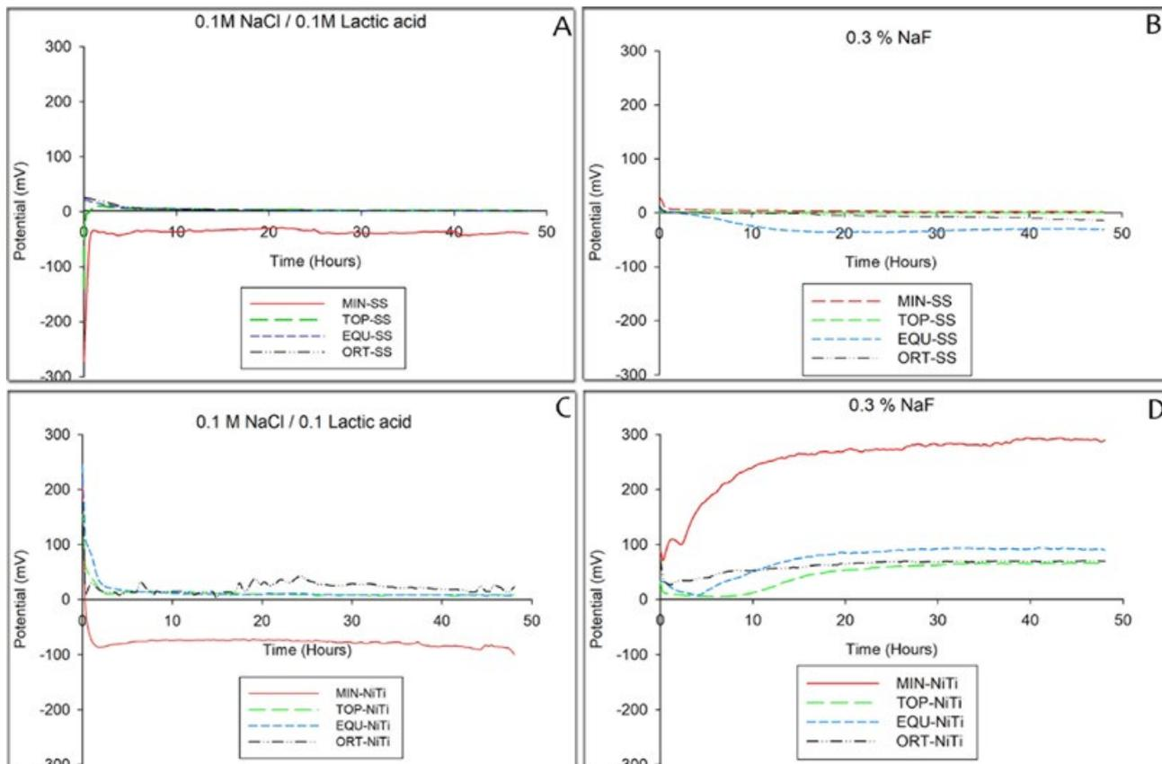
Figure 2. Representative curves from all bracket wire combinations tested showing the potential difference over time for both solutions. A and B depict the curves of bracket-SS wire combinations for 0.1 M NaCl -0.1 M lactic acid solution and 0.3% NaF respectively. C and D show the curves for bracket-NiTi wire combinations.
