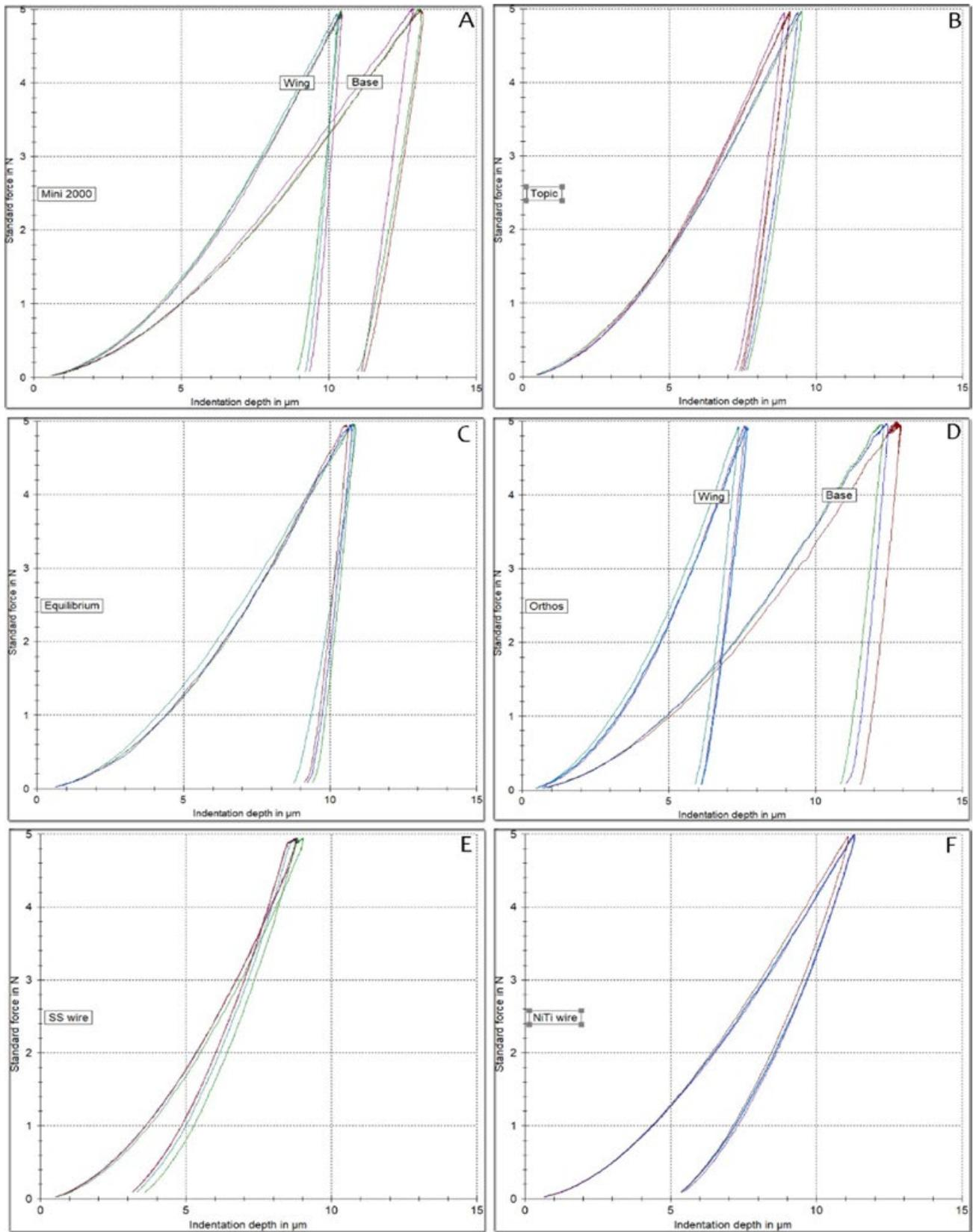
Figure 1. Representative force indentation curves from all materials tested. MIN (1A) and ORT (1D) demonstrate big difference in relative curve position for base and wing regions while TOP (1B) and EQU (1C) provide almost identical curves from both regions. The curves of SS (1E) and NiTi wire (1F) are also presented.
