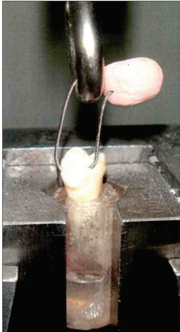
Figure 1. Bonded specimen loaded in the Instron machine.
