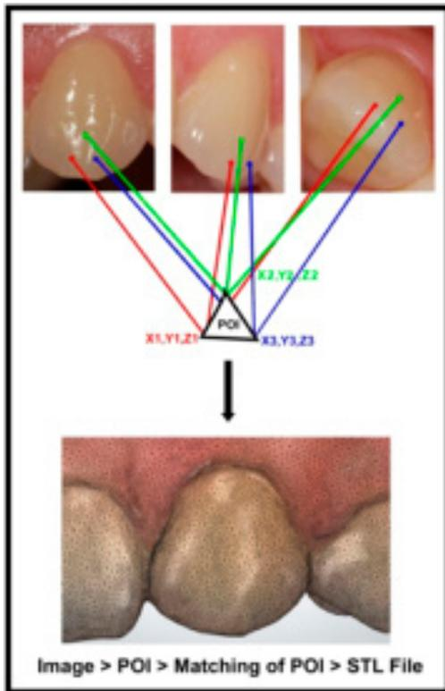
Figure 1. Image acquisition mechanics of the IOS devices.
