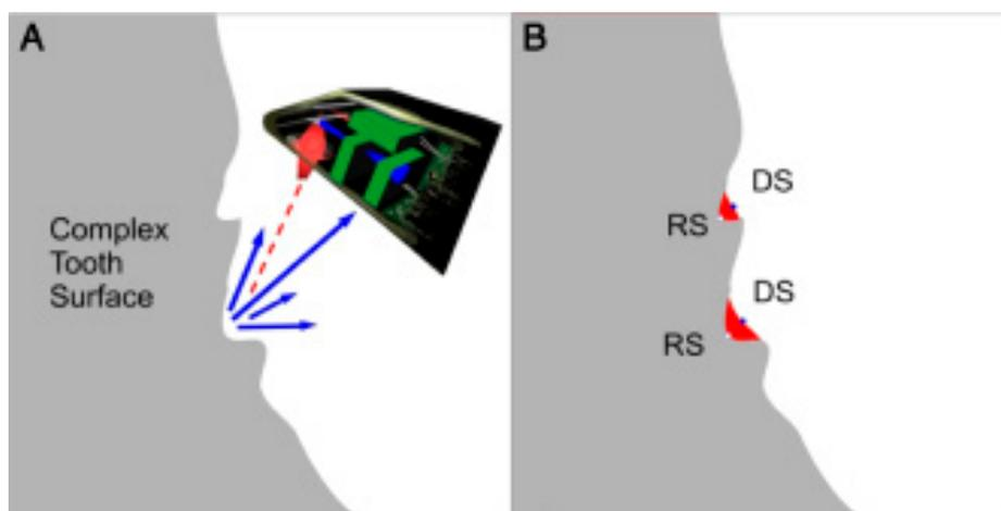
**Figure 7.** A: Behavioural differences of light reflected from complex surfaces B: Schematic illustration of the flattening occurring on complex surfaces, RS: Real surface and DS: Virtual surface obtained in the digital model.
