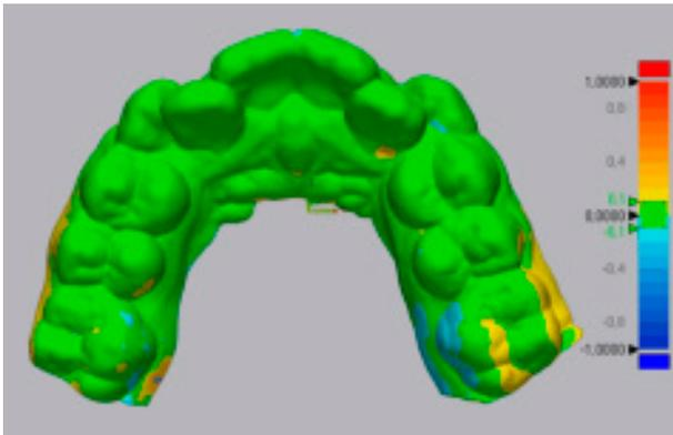
Figure 6. Overlapping of the VAs. The meanings of the color codes: green; perfectly aligned areas, red; positively positioned areas (PPA) relative to the reference model, blue; negatively positioned areas (NPA).
