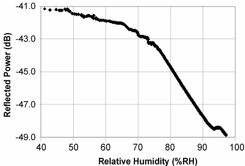
Figure 7. Response of the sensor to relative humidity variations.
