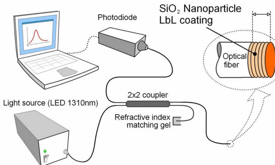
Figure 5. Fiber optic sensor experimental setup.
