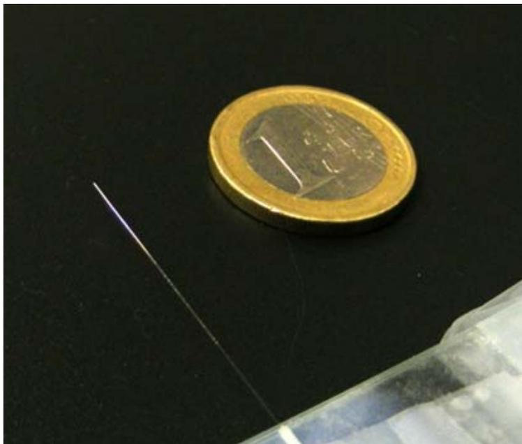
Figure 4. Picture of the nano-Fabry- Perot sensor.
