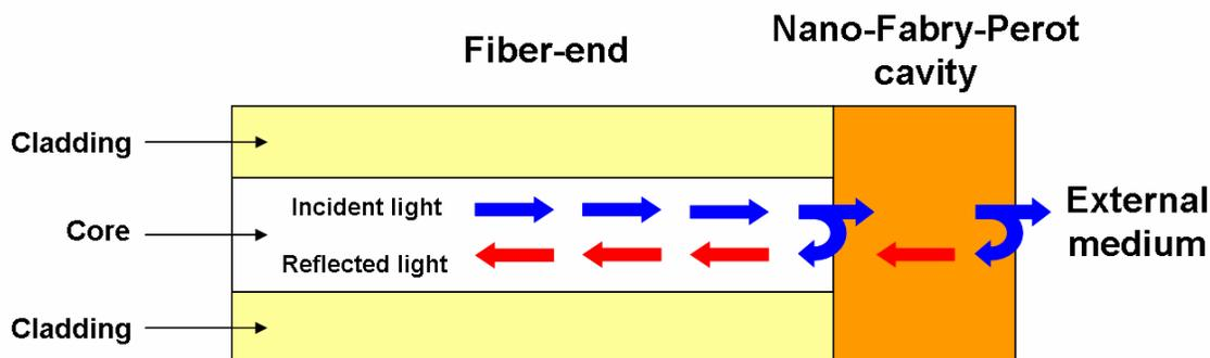
Figure 3. Schematic of the Nano-Fabry-Perot cavity coated on a perpendicularly cleaved fiber optic tip.
