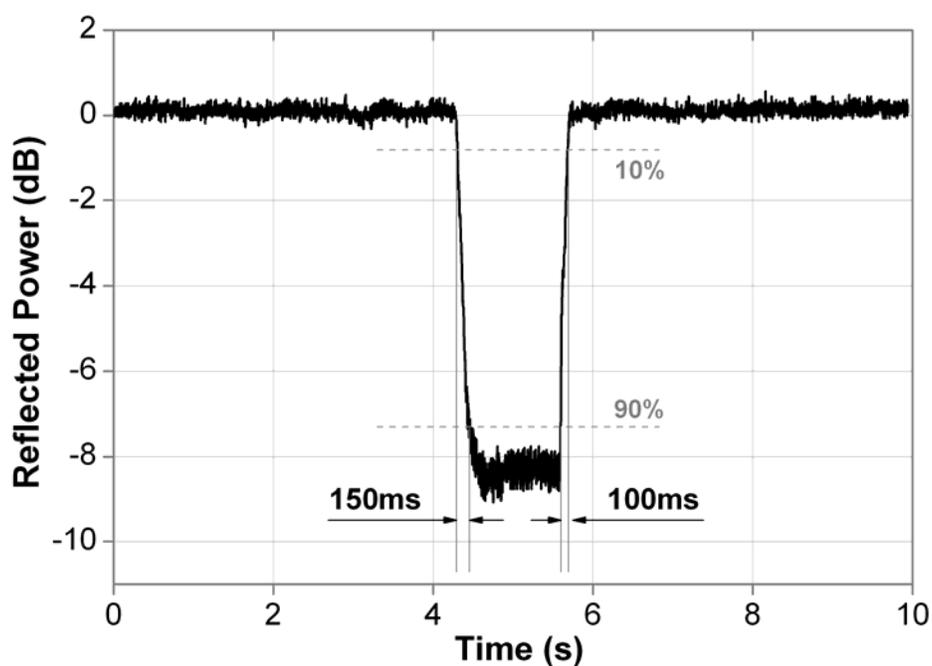
Figure 8. Dynamic response of the sensor to a breathe exhalation. Rise and fall times are displayed in the graphic.
