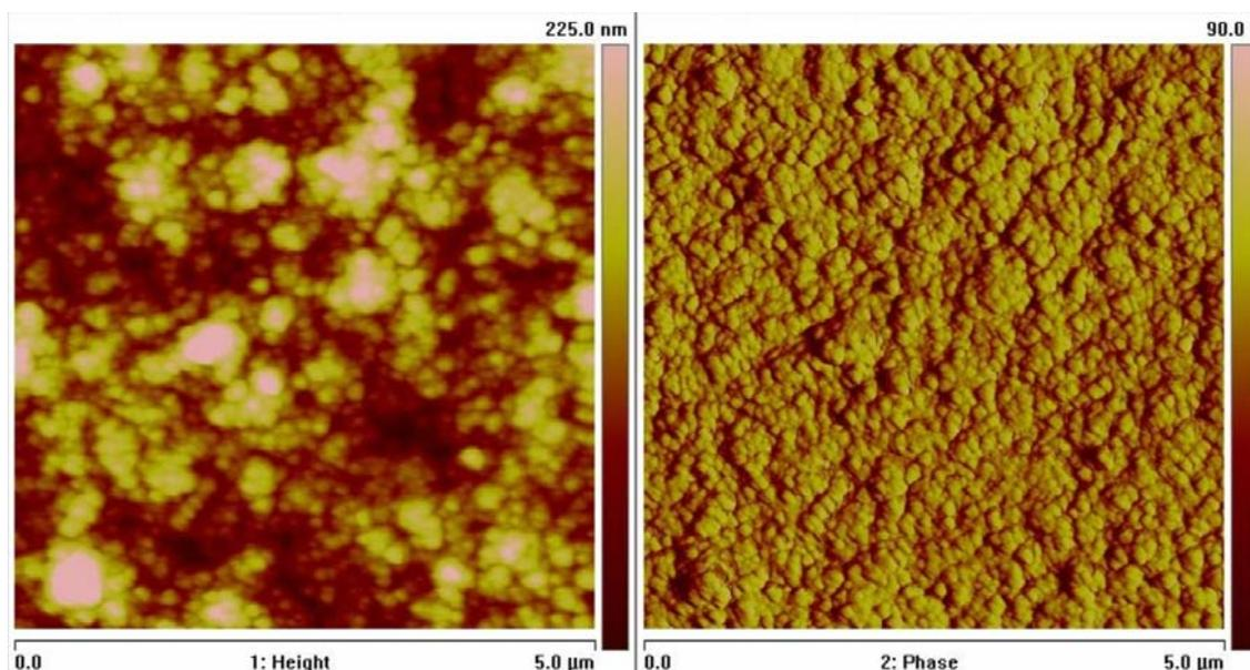
Figure 1. AFM height and phase images of a film with 23 bilayers of SiO<sub>2</sub> nanoparticles.
