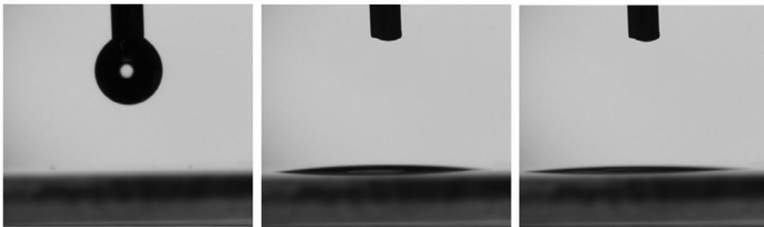
Figure 2 Photograph sequence of the contact angle of a water droplet on a superhydrophilic LbL nanostructured coating. a) Before touching the surface. b) After 0.5 seconds. c) After 1 second.
