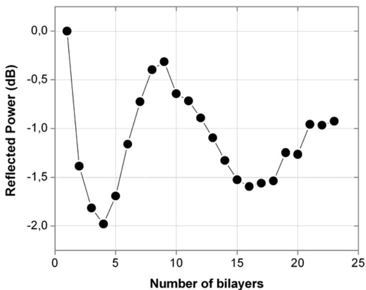
Fig.6. Reflected optical power while the coating was built-up.
