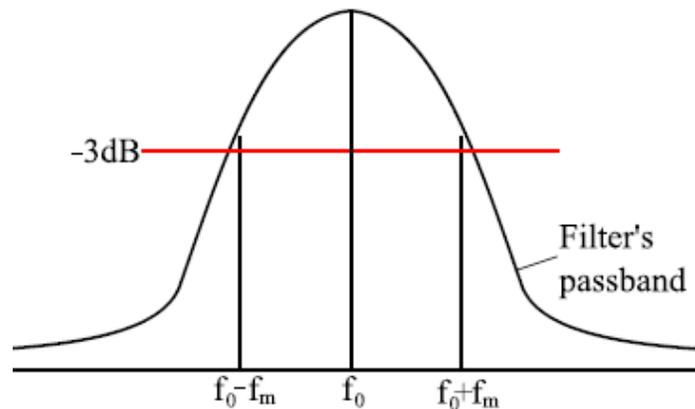
Fig. 8. ASK-keyed signal sidebands and Q value
