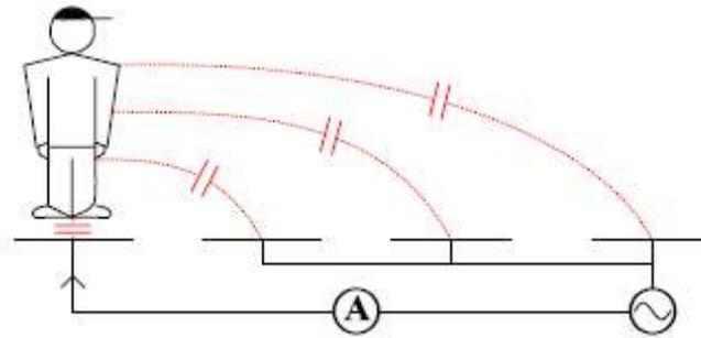
Fig. 1. The current flow of a single element is affected by a person. The whole element matrix is scanned sequentially.
