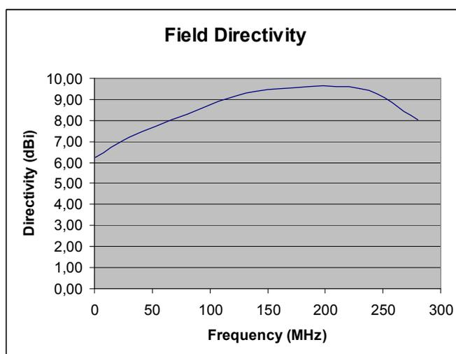
Fig. 6. Field directivity of the quad antenna
