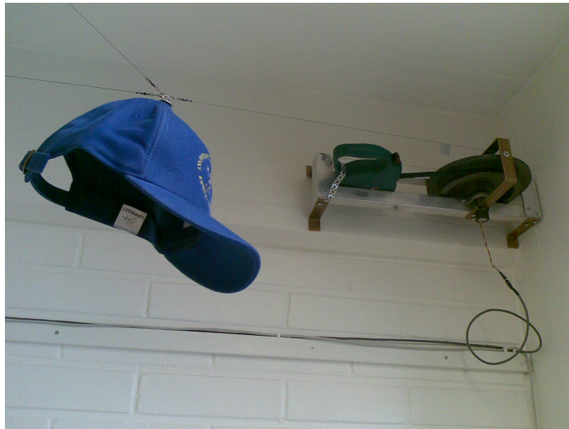
Figure. 1. The triangulation reference reel and the positioning hat. Retractable dog leashes are used to achieve the retracting motion of the positioning lines. The ten-turn precision potentiometer used is visible under the spool on the right.
