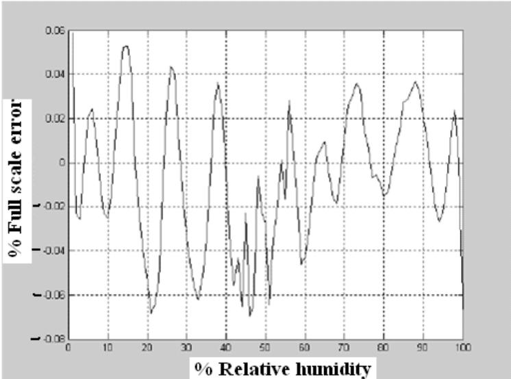
**Fig. 7. % Full scale error curve for Relative Humidity**
