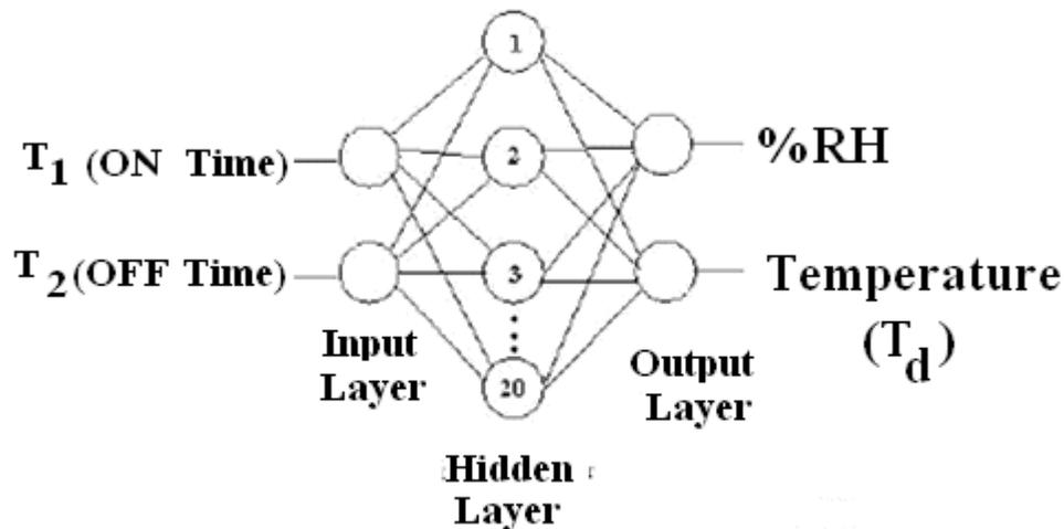
**Fig. 6. ANN structure used as Lineariser**
