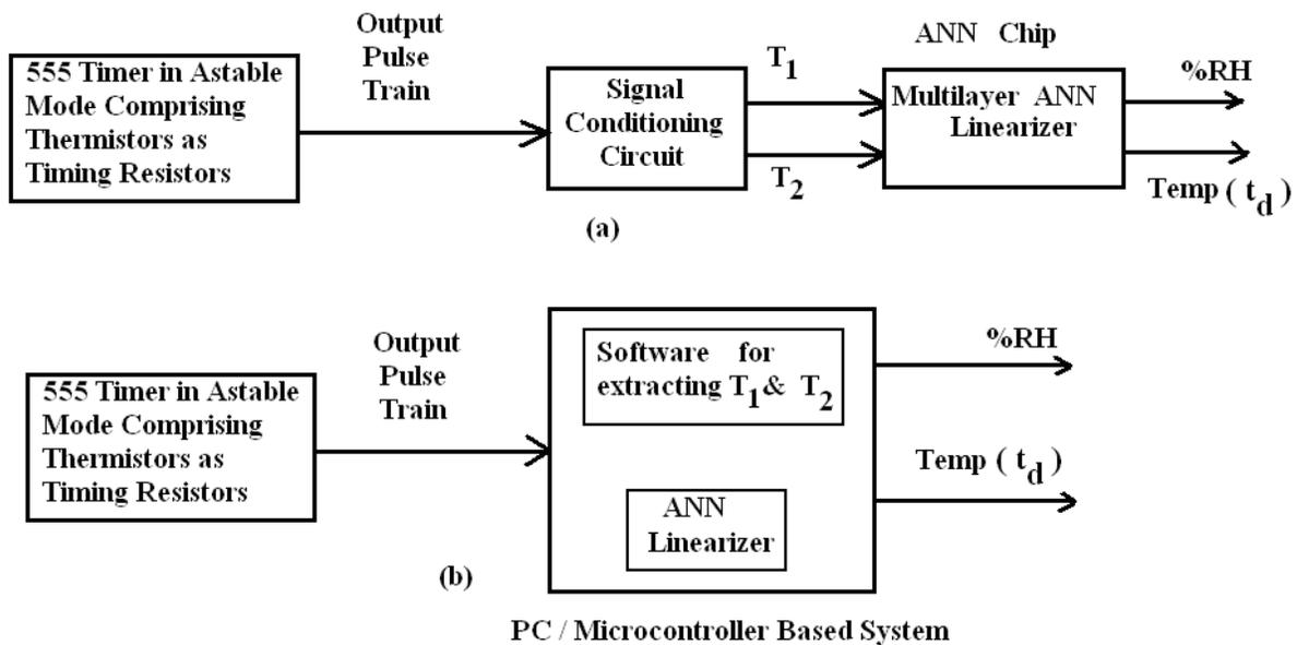
Fig. 5. Block Diagram Representation of the Proposed Scheme
