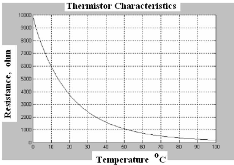
Fig.3. Resistance vs. Temperature characteristics of Thermistor
