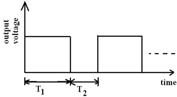
Fig. 2. Output waveform of 555 timer in astable mode
