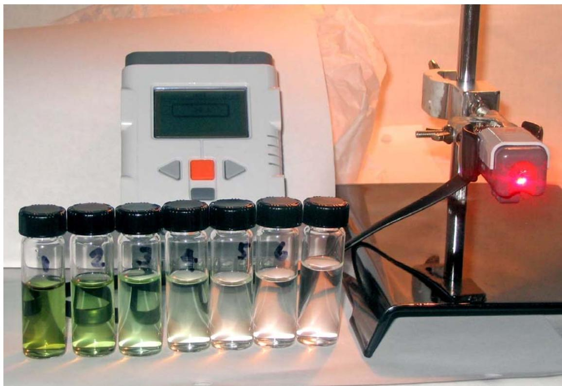
*Figure 1. The Lego Mindstorms NXT™, 9844 optical sensor, ringstand, clamp and solutions used in the experiment are shown. A silvered mirror and 1 cm glass cuvette are not shown.*
