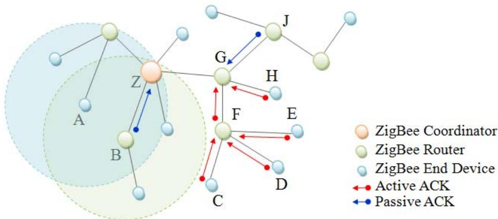
Figure 2. ZigBee tree-based network topology
