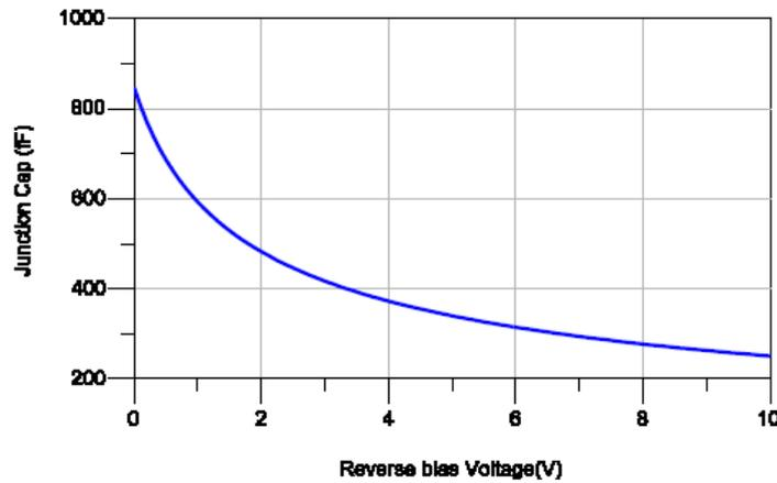
Fig. 3. Junction capacitance vs. reverse-bias voltage for the chosen CMOS technology
