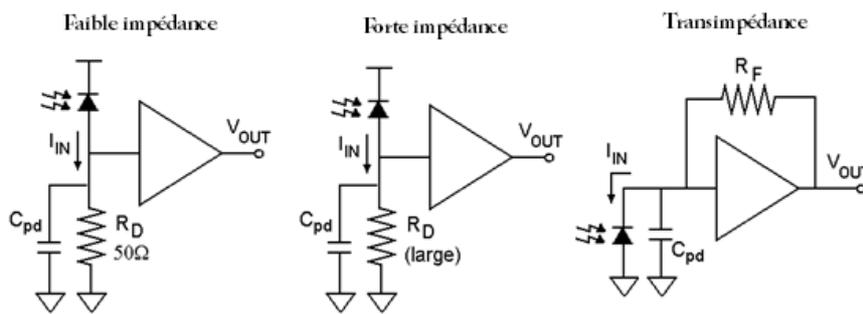
Fig. 5. Preamplifier configuration
