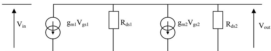
Fig. 6.b Push-Pull inverter equivalent circuit
