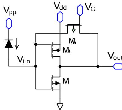
Fig. 7. Original 3-Transistor design for preamplifier stage
