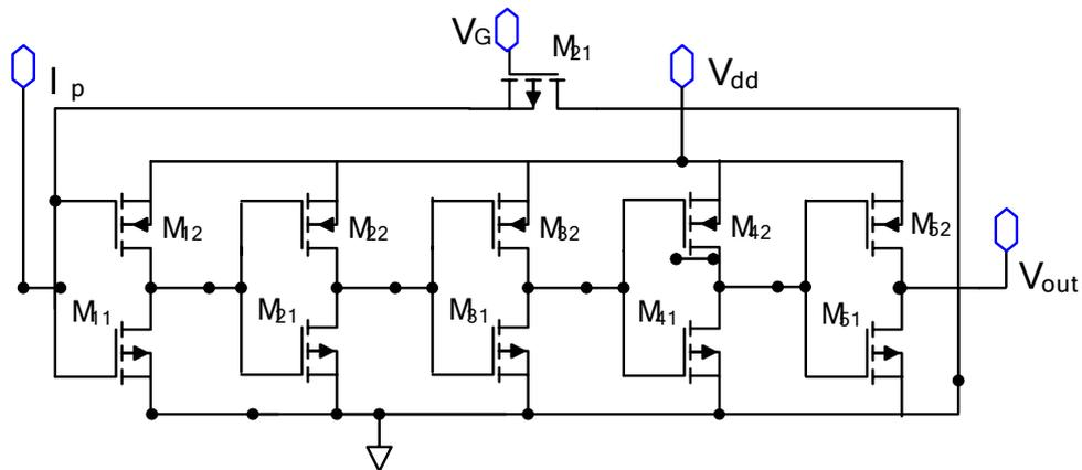
Fig. 8. The CMOS transimpedance amplifier without series peaking TIA optimization
