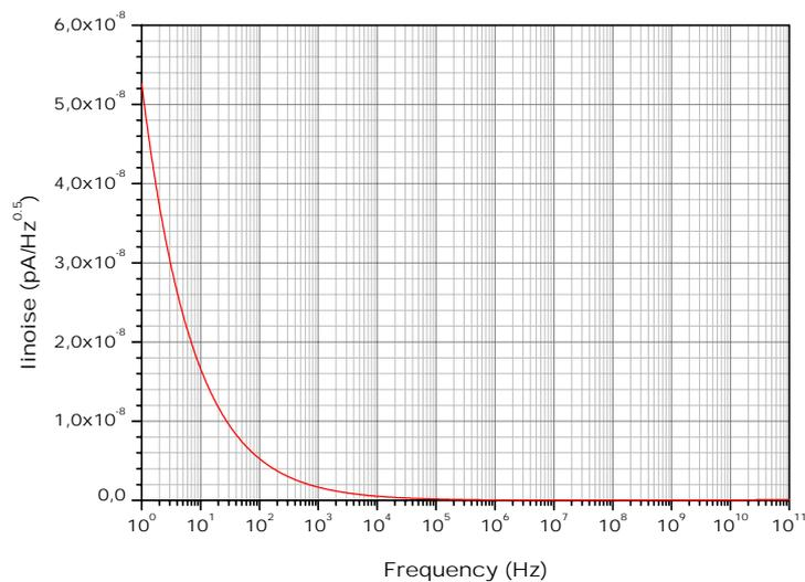
Fig. 11. Input noise current of the transimpedance
