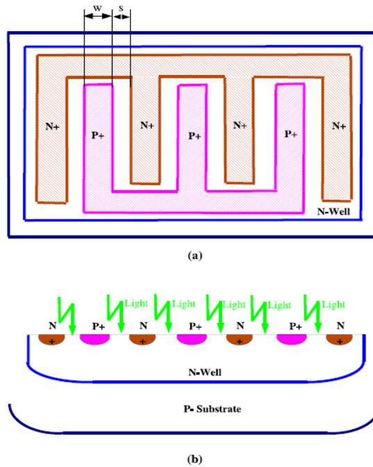
Fig. 2. Photodiode implemented in AMS C35 (a) top view of the interdigitated photodiode (b) cross-section of the photodiode.
