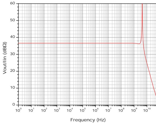
Fig. 10. The transimpedance gain of the preamplifier.
