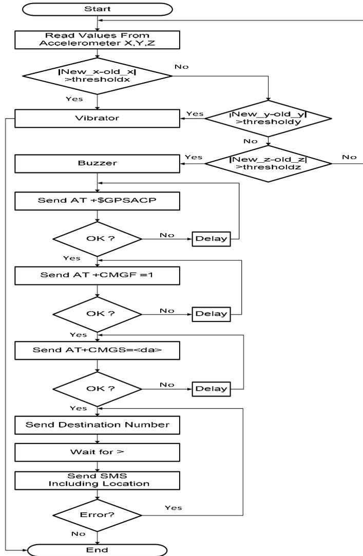
Figure 7. Flow Chart for Reading Accelerometer Sensor.
