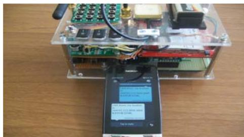
Figure 9: Testing GSM-GPS Module and Accelerometer Sensor.
