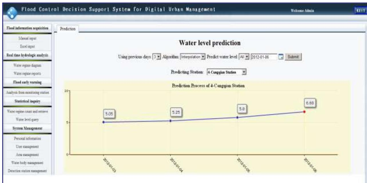
Figure 8. The result of predicting the water level using the interpolation method
