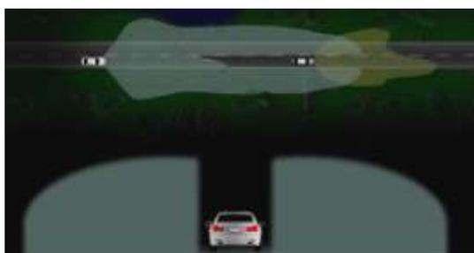
Figure 9. Principle of BMW's Matrix-LED
