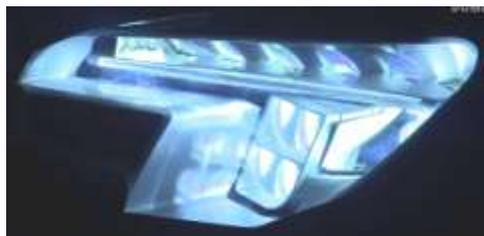
Figure 6. Matrix-LED lamp from Opel
