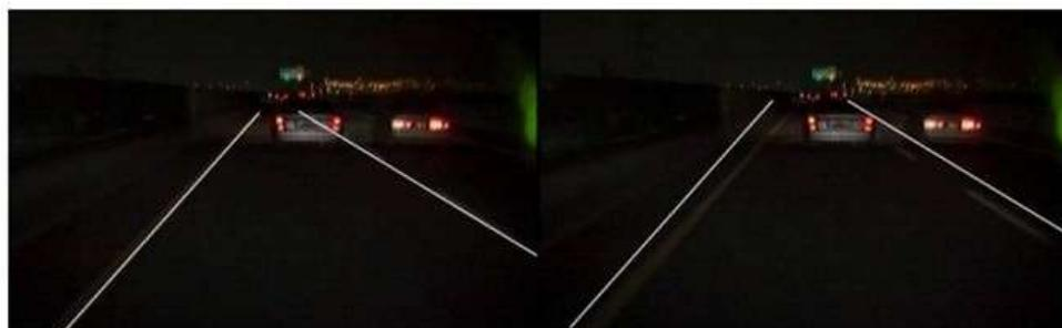
Figure 24. Lane information merged vehicle lights detection without and with offset [14]
