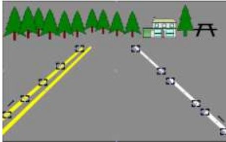
Figure 14. Feature based lane marking detection
