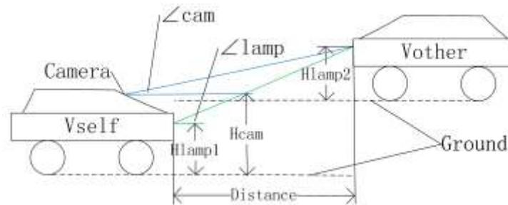
Figure 28. Horizontal headway calculation
