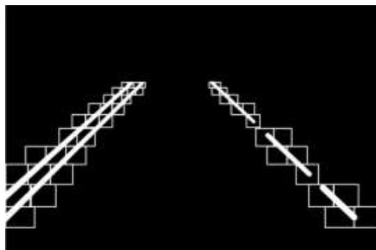
Figure 12. Pick out interested windows that include lane markings
