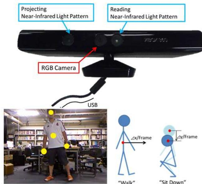
Figure 2. Kinect Sensor
