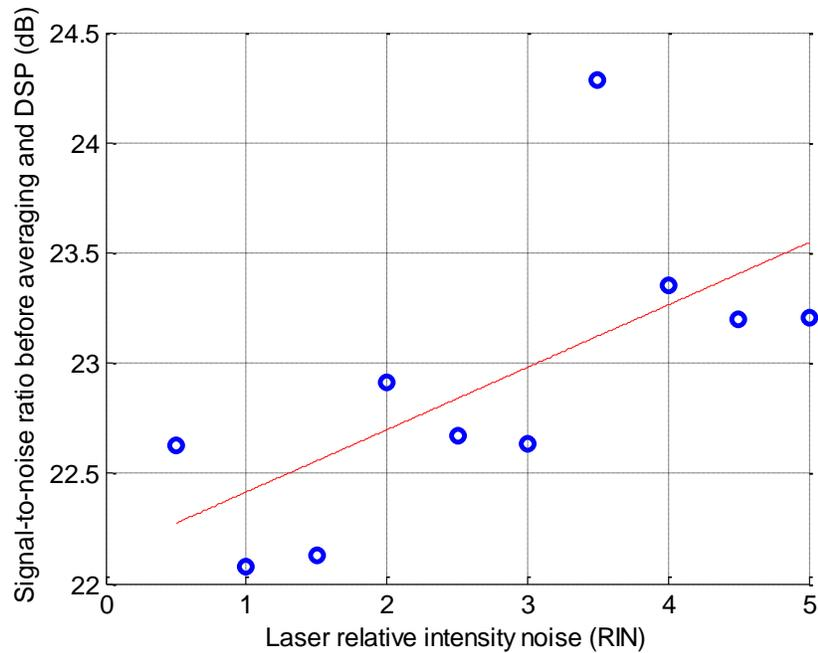
Figure 4: SNR as a function of laser RIN (%) for a BOTDA system.
