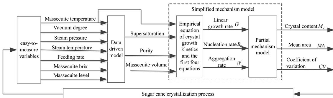
Figure 6. Overall scheme for the hybrid modeling in sugar cane crystallization
