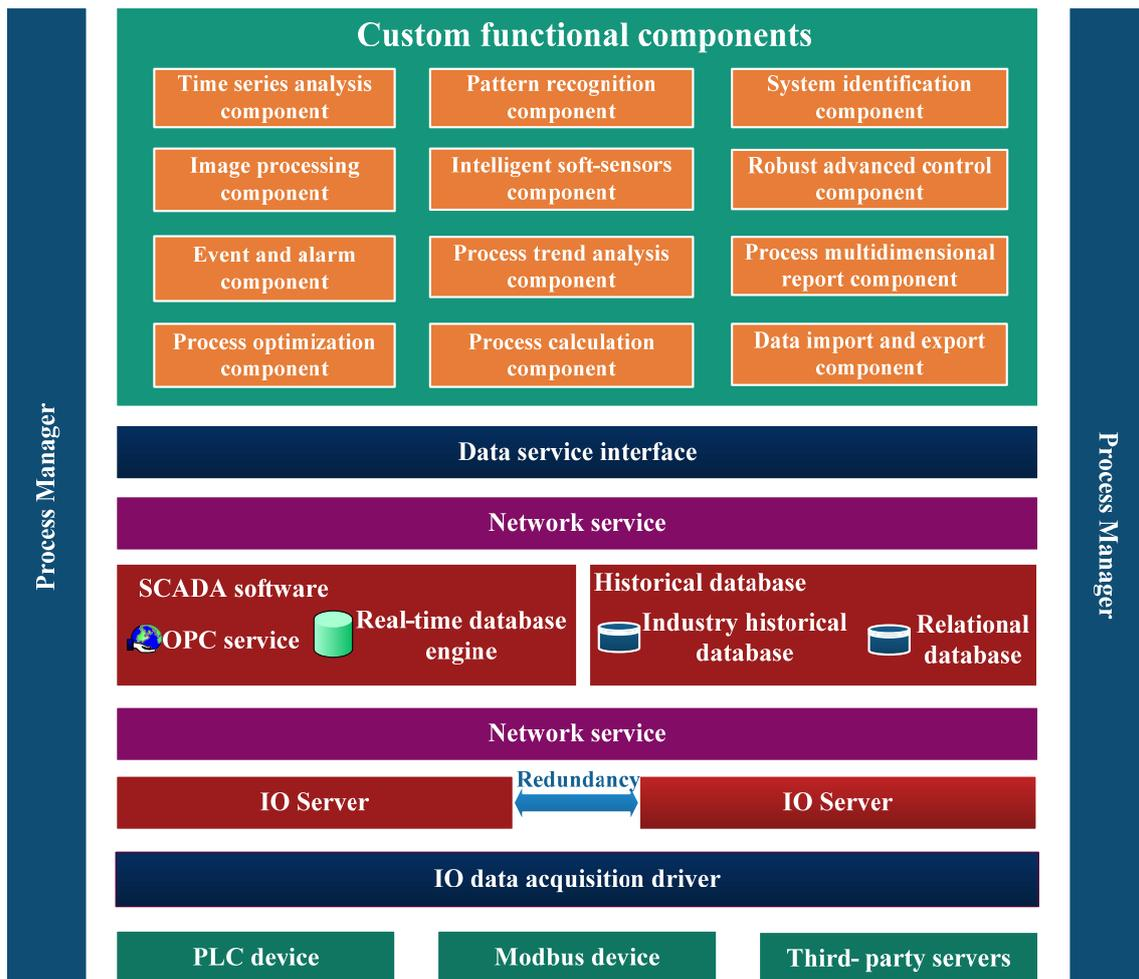
Figure 2. The software architecture of intelligent integrated measuring and control system for sugar cane crystallization process
