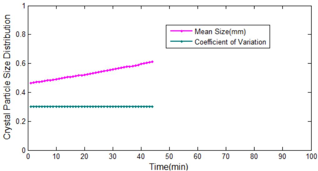
Figure 12. On-line prediction of CSD for sugar crystallization
