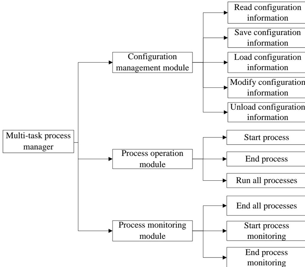
Figure 3. Architecture of the multi-task process manager for sugar cane crystallization process
