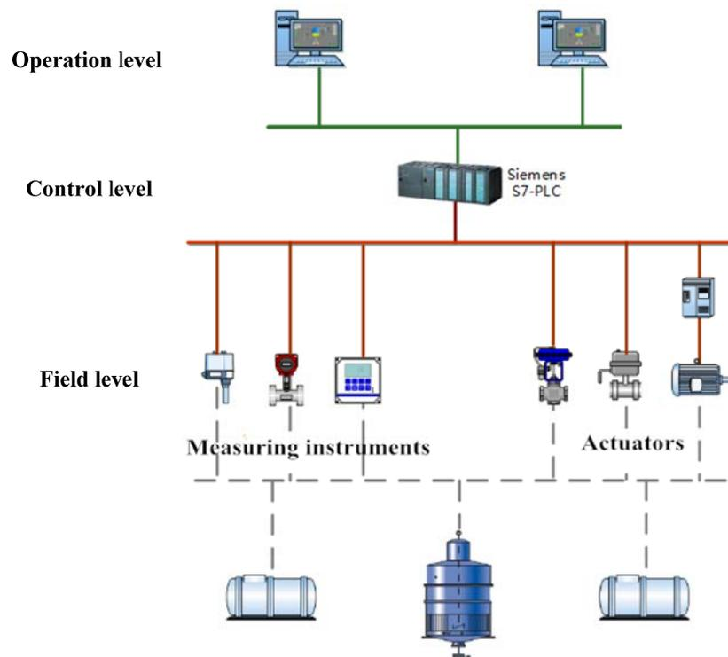
Figure 1. The hardware architecture of intelligent integrated measuring and controlling system for sugar cane crystallization process
