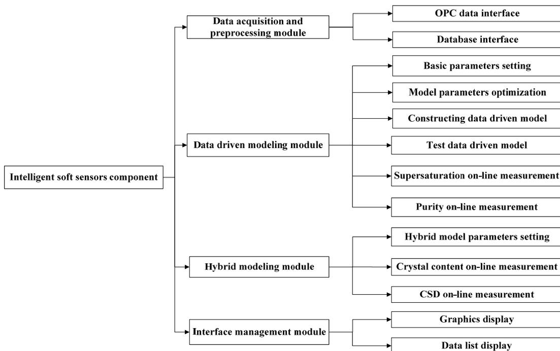
Figure 5. Architecture of soft-sensors component for sugar cane crystallization process
