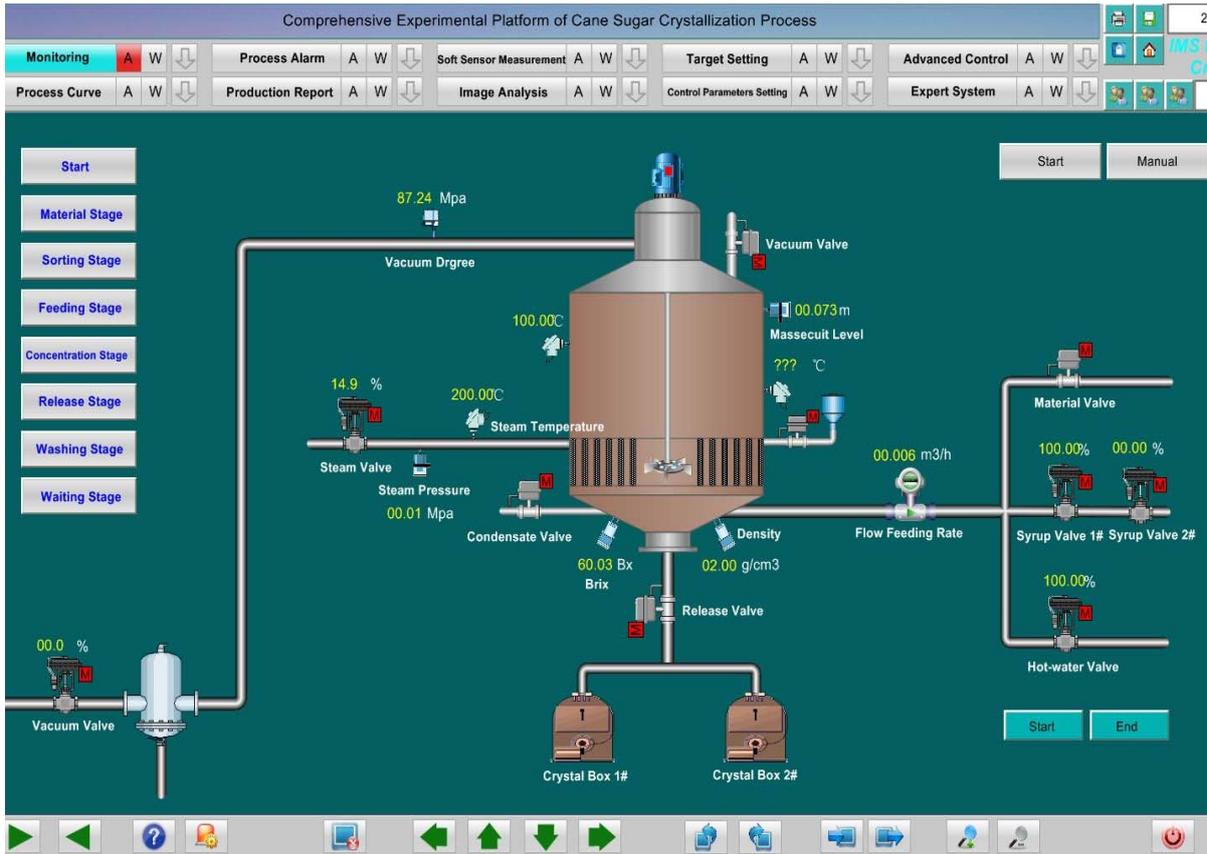
Figure 4. Main interface of process monitoring system
