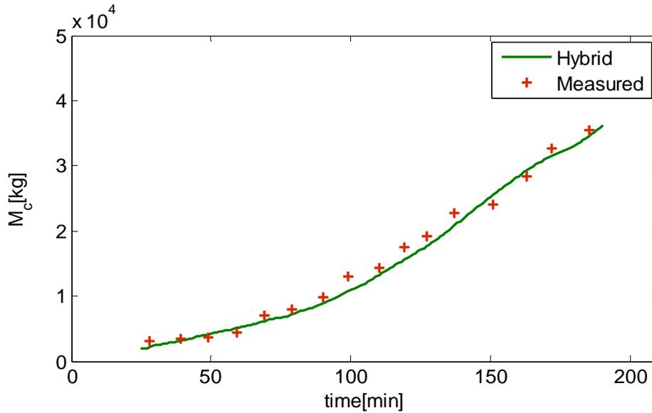
Figure 11. On-line prediction of crystal content for sugar cane crystallization
