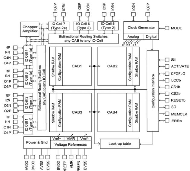
Figure 3: Internal block diagram of FPAA (Anadigm FPAA).
