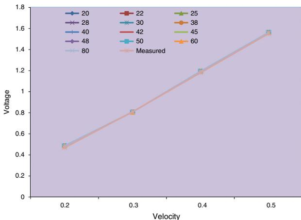
Figure 9: MEMS seismic sensor characteristics—velocity v/s output voltage of after vibrating frequency compensation.
