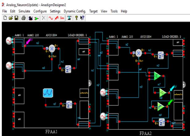
Figure 5: Implementation of FPAAs based interface circuit in anadigm designer 2.
