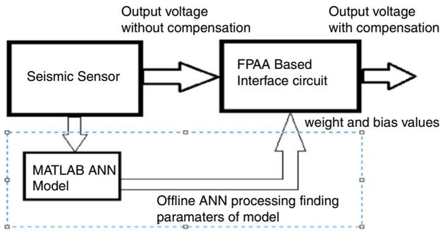
Figure 4: Block diagram of sensor with FPAAs based interface circuit.
