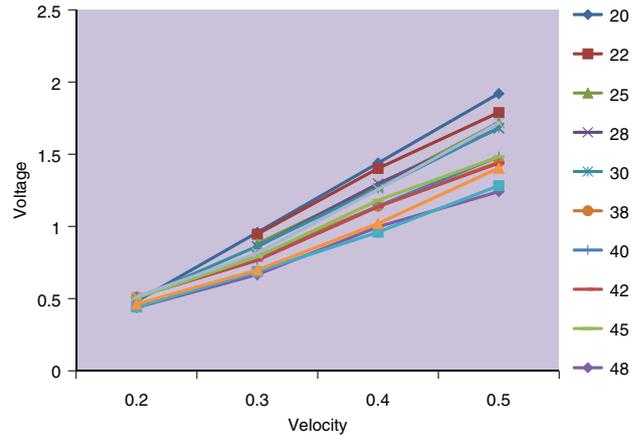
Figure 1: MEMS seismic sensor characteristics—velocity V/S output voltage of before vibrating frequency compensation.
