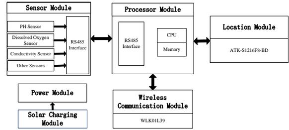
Figure 2. Water quality monitoring node hardware block diagram
