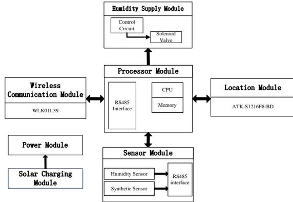
Figure 4. Hardware Block Diagram of Soil Monitoring Node
