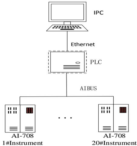
Figure 1. Detection system network structure
