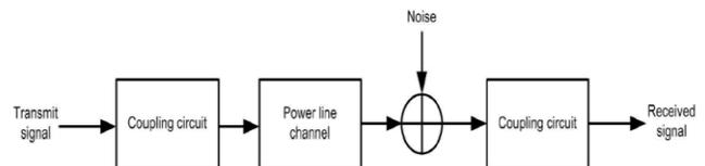
Figure 1. Graphical illustration of the PLC channel
