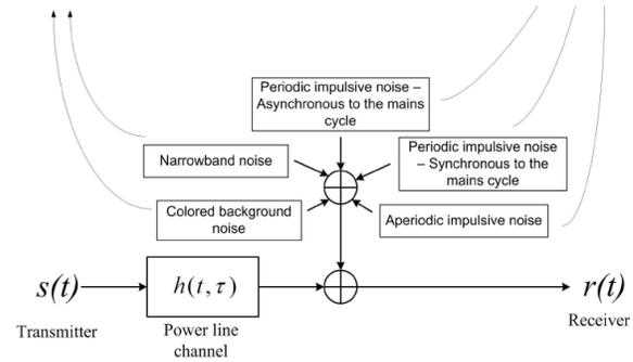
Figure 2. Noise Type observed in PLC systems
