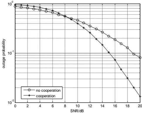
Figure 2. outage probability of cooperation system and no cooperation system with the SDF cooperation model
