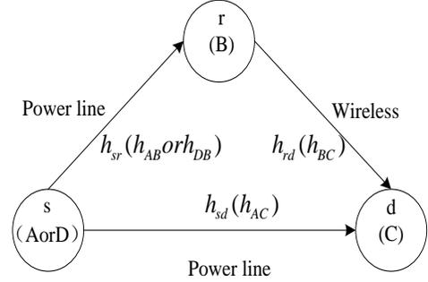
Figure 1. Basic structure of proposed PLC system
