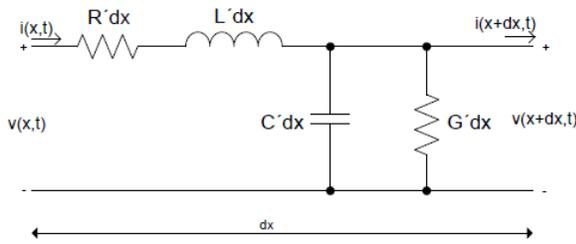
Figure 1. Elementary cell of a transmission line
