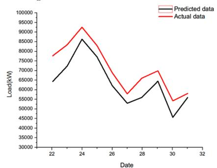
Figure 4. Predicted load by GA-BP network and actual load
