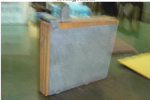
Fig. 2 cathode plates are arranged in an alternating arrangement
