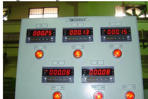
Fig. 14 Another resistance value of the soldering points are shown in meter
