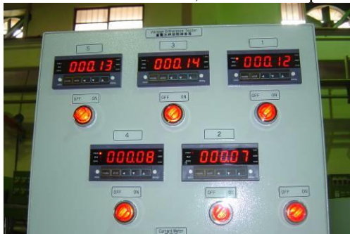
Fig. 13 The resistance value of the soldering points are shown in meter
