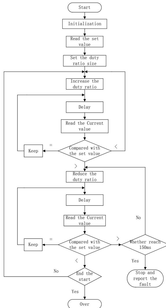
Figure.9 Flow chart of current limiting soft start
