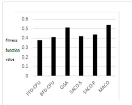
Figure.5 Comparison of the fitness function value of 6 kinds of placement algorithms
