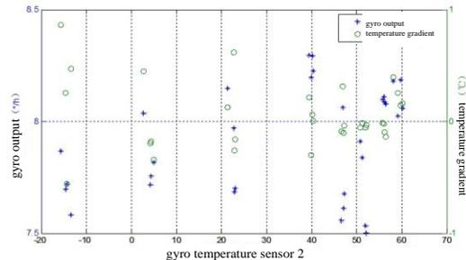
Figure 5. Relationship between temperature gradient and gyro zero bias
