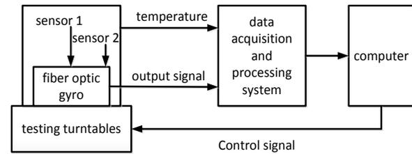
Figure 1. Equipment connection about temperature test
