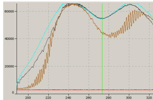
Figure 2. The absorption spectrum of  $SO_2$  and  $NO_2$
