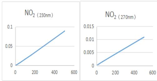
Figure 4. Data relationship between concentration and absorbance of NO<sub>2</sub>.
