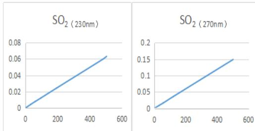
Figure 5. Data relationship between concentration and absorbance of SO<sub>2</sub>.
