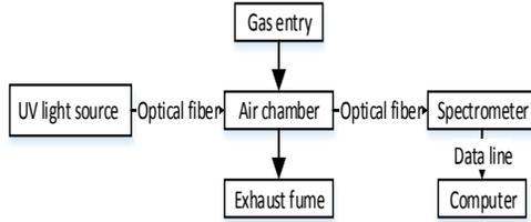
Figure 3. Flow chart of the experimental system.
