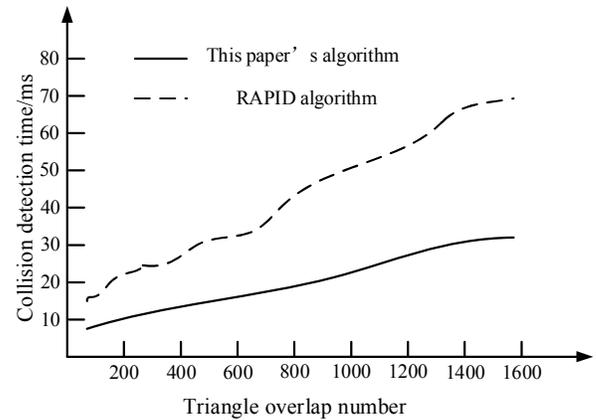
Figure 4. Time contrast diagram of algorithm collision detection
