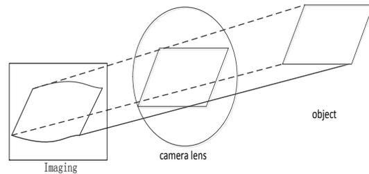
Figure 4. Radial distortion
