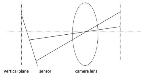
Figure 5. Tangential distortion
