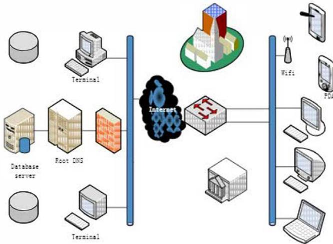
Figure 11. IPV9 root domain name proxy system topology
