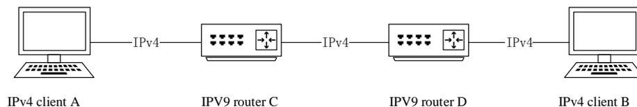
Figure 8. IPv4 network test topology through 9over4 tunnel connection
