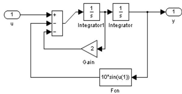
Figure 1. Simulink Block Diagram of Mechanical Arm
