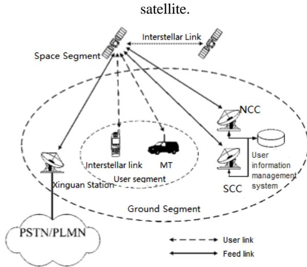
Figure 1. Basic composition of satellite communication link
