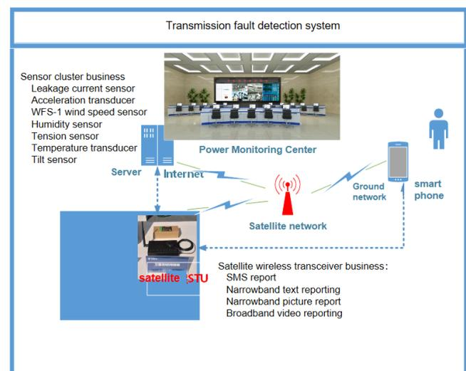
Figure 4. The logic diagram of the high-level scheme of the transmission fault monitoring system
