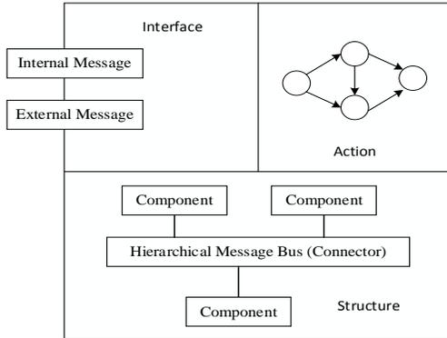
Figure 2. Component model of HMB architecture
