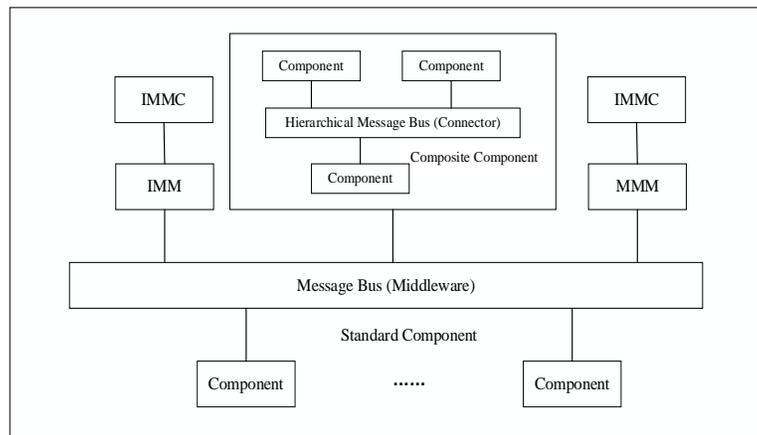
Figure 4. Schematic diagram of the NHMB architecture
