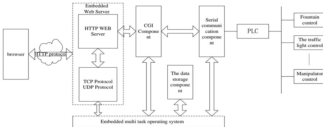
Figure 3. Structure diagram of software system
