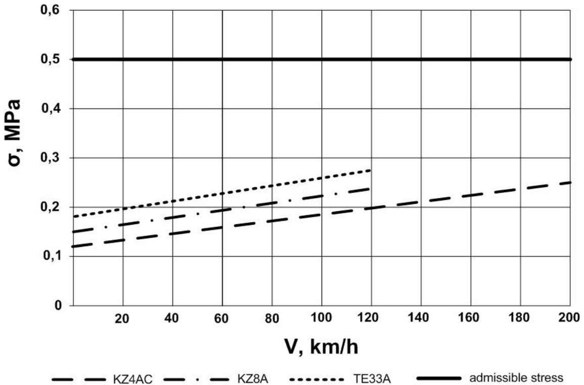
Fig. 4. Stress in ballast layer under rails
