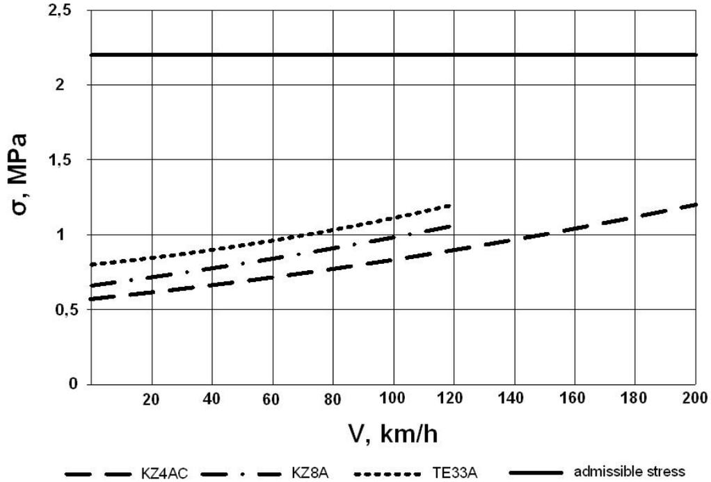
Fig. 3. Stress under rail bearing plates
