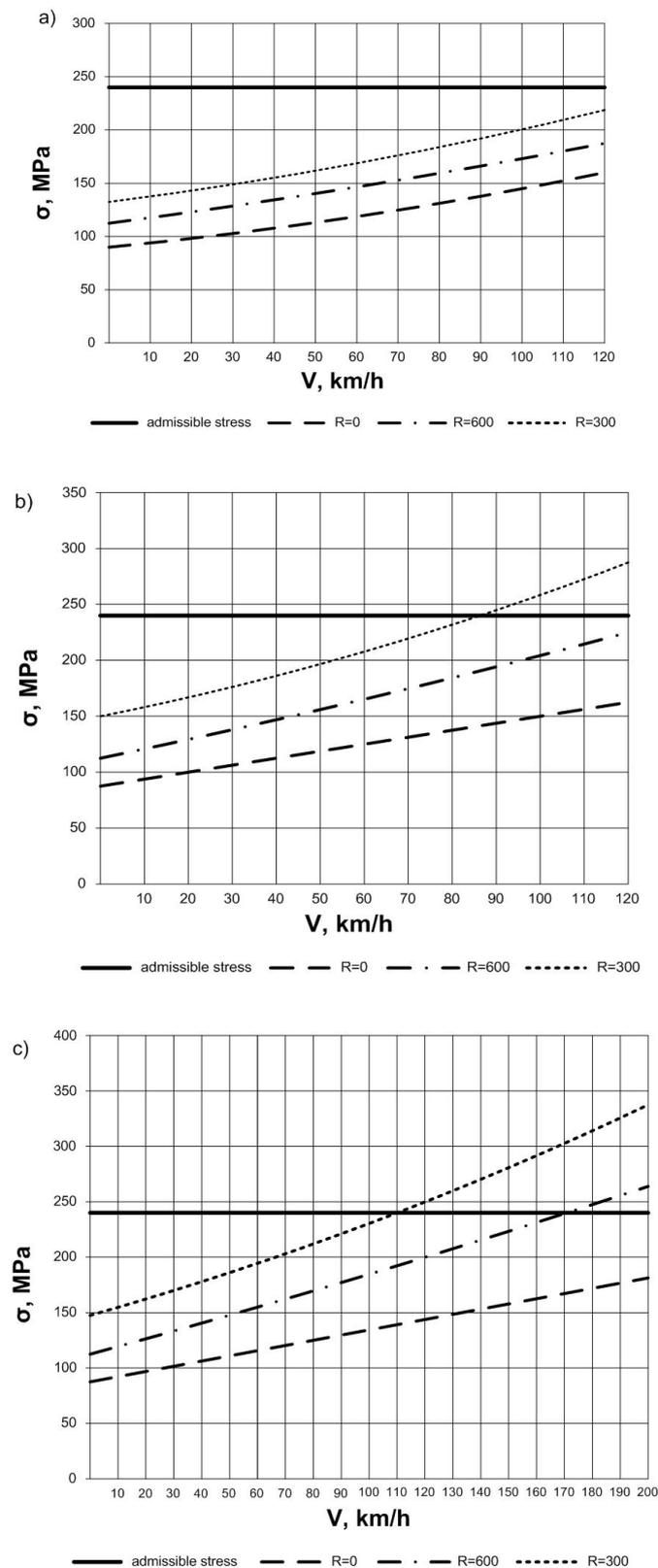
Fig. 2. Stress in the edges of rail foot in tangent ( $R=0$  m) and curved track ( $R=600$  m,  $R=300$  m) under locomotives operation: KZ8A (a), TE33A (b), KZ4AC (c)
