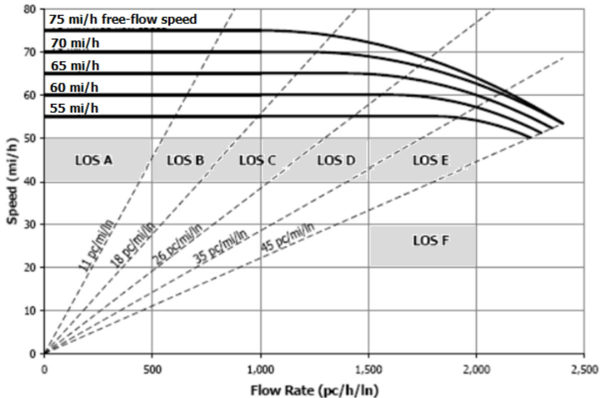
Fig. 3. Speed Flow Curve on basic freeway segments as per HCM 2010
