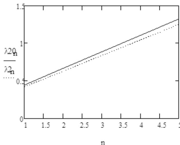
Fig. 3. Diagram of changes in Eigenfrequency under bending vibrations (in harmonics) for a standard frame  $\lambda_{20n}$  and a modernized one (with damping bottom covering)  $\lambda_{2n}$  for the first and the third section of the frame of emergency and repair rail service car
