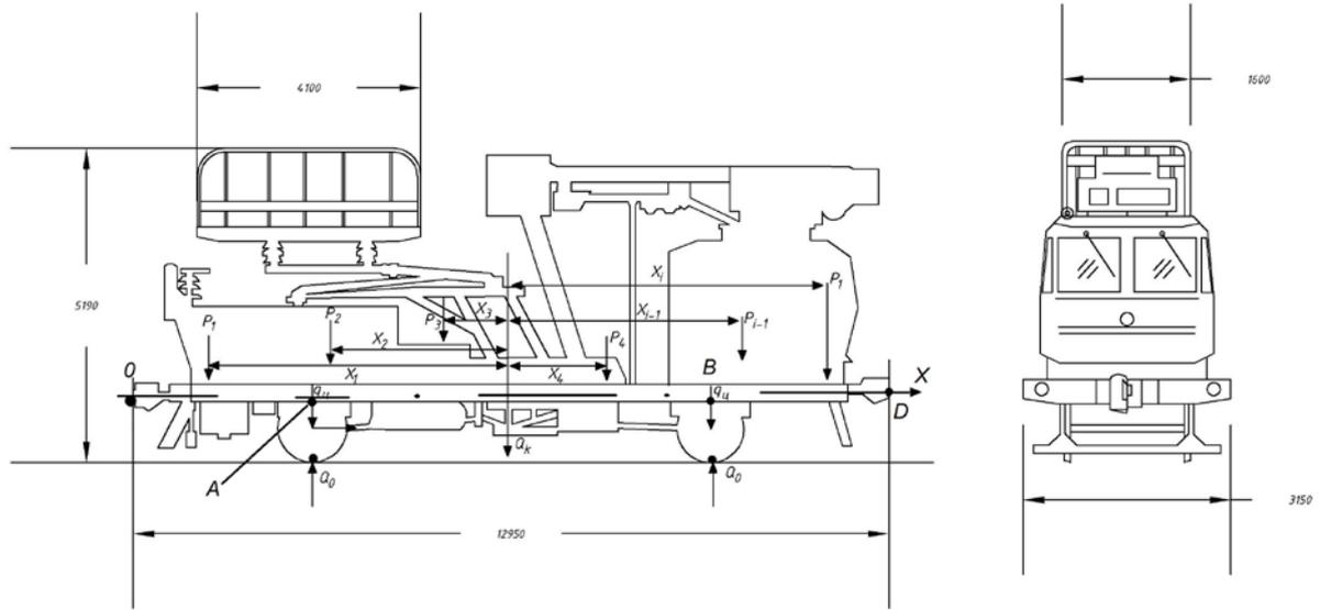
Fig. 1. Design scheme of the rail car for the equivalent load-bearing frame of the body frame
