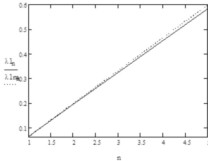
Fig. 2. Diagram of the change in eigenfrequency under longitudinal vibrations (in harmonics) for a standard frame  $\lambda_{1n}$  and a modernized one (with damping bottom covering)  $\lambda_{1m_n}$ .
