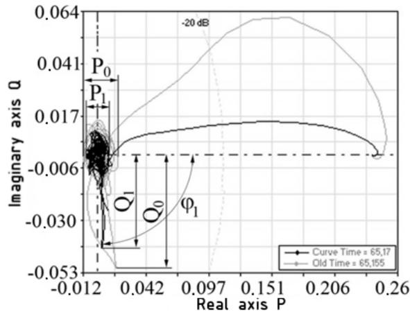
Fig. 6. Amplitude and phase-frequency characteristics at vanishing of sliding velocity
