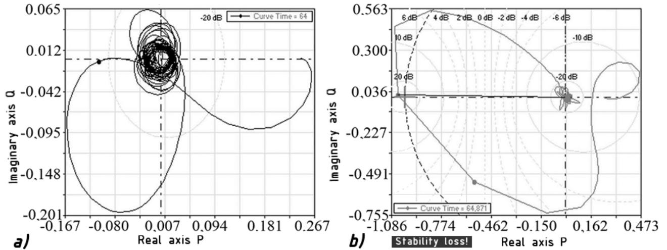
Fig. 5. Amplitude and phase-frequency characteristic of tribosystem instability: a - development of frictional jumping; b - stability losses on amplitude (an inertial component)
