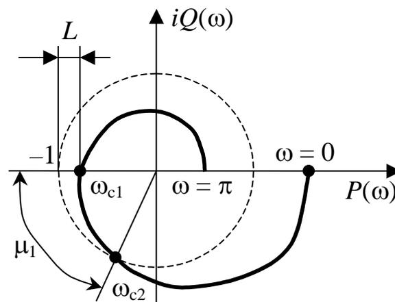
Fig. 4. Illustration of the stability factor on amplitude and phase
