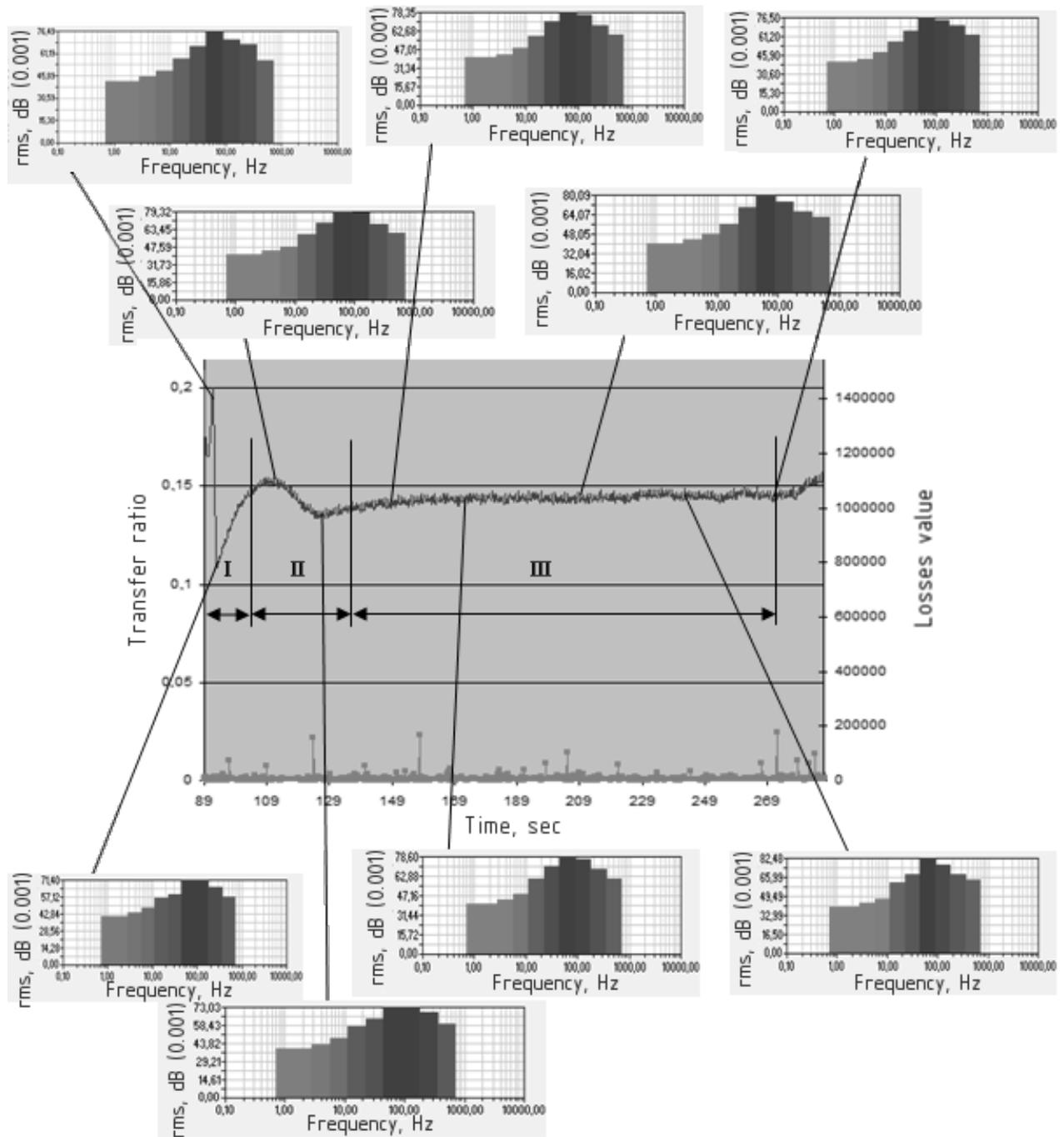
Fig. 3. Application of FSMA as a grease: I - area of spraying, II - area of distribution of material, III - area of work
