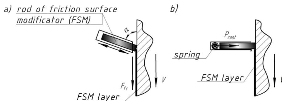
Fig. 1. The scheme of contact-rotaprint modification of friction surfaces: a) drive gear on the base of servoeffect; b) conventional drive gear
