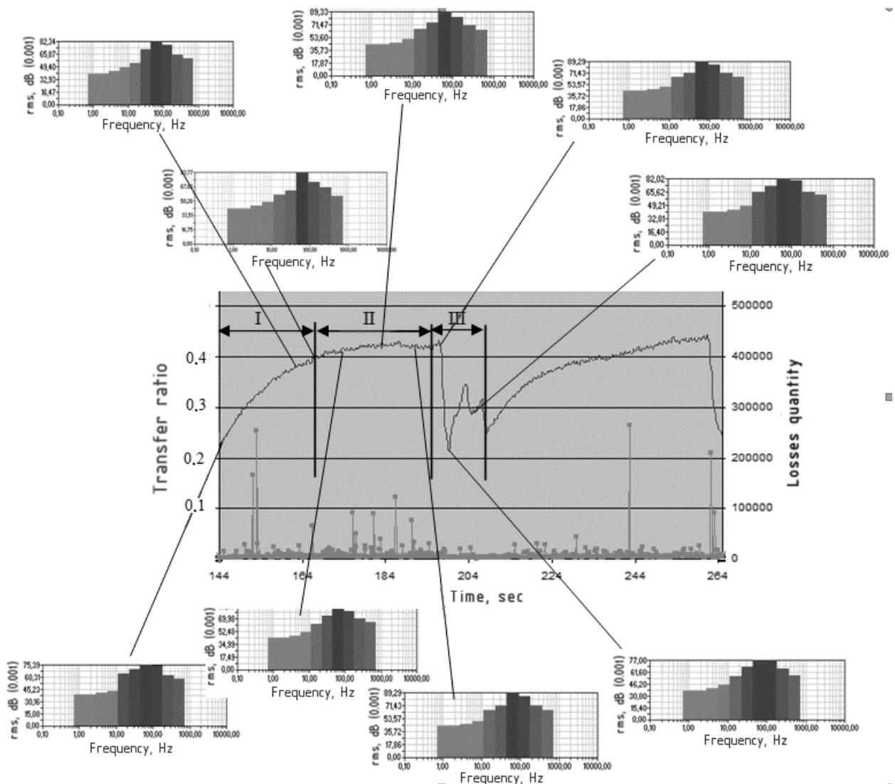
Fig. 2. Application of FSMA to tractive effort increase: I - area of spraying, II – area of work, III - area of cleaning of friction surface
