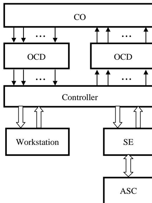
CO – is a controlled object; OCD – is the object communication device; SE – is switching equipment; ACS – is an automated control system of the highest level.
