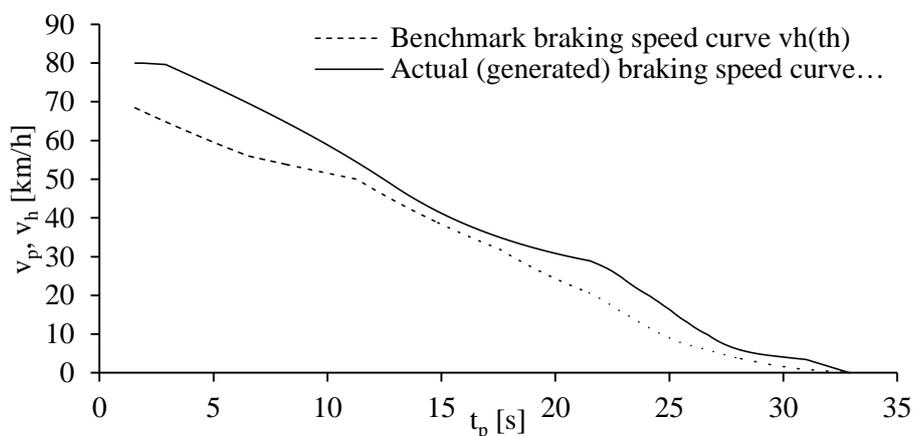
Fig. 9. Implementation of the braking curve for the selected station for initial braking speed  $v_p=80$  km/h
