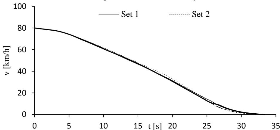
Fig. 5. Trajectories of braking speed depending on the adopted controller parameters (parameters of terms of a controller); the degree of filling  $st=1,0$ ; speed of initiation of braking  $v_p=80$  km/h, and the complex route profile
