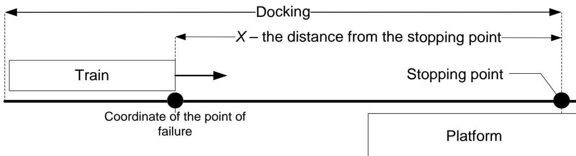
Fig. 7. Approaching section of the selected station in front of which the failure of the propulsion system of one car occurs
