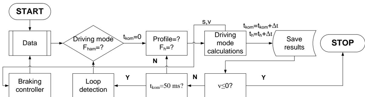
Fig. 4. A general block diagram of the simulation model—functional scheme
