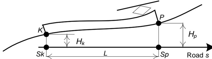
Fig. 3. A train on a facultative geodesic profile of the track—a simplified method of determining a replacement profile
