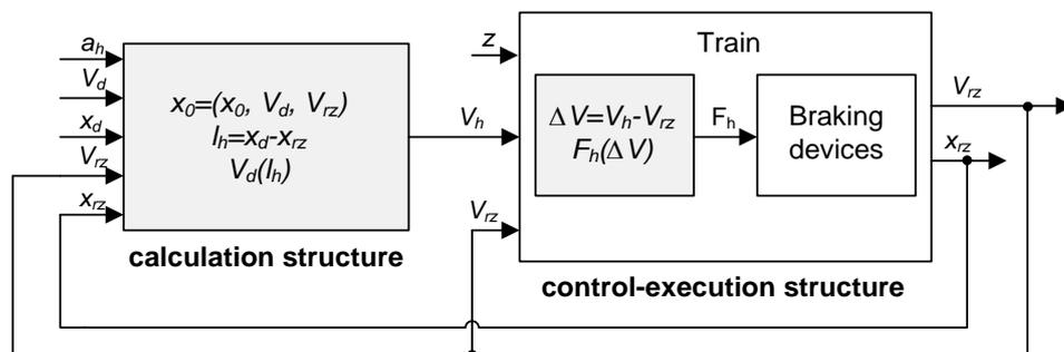
Fig. 2. Structure of the automatic braking system [1, 4]
