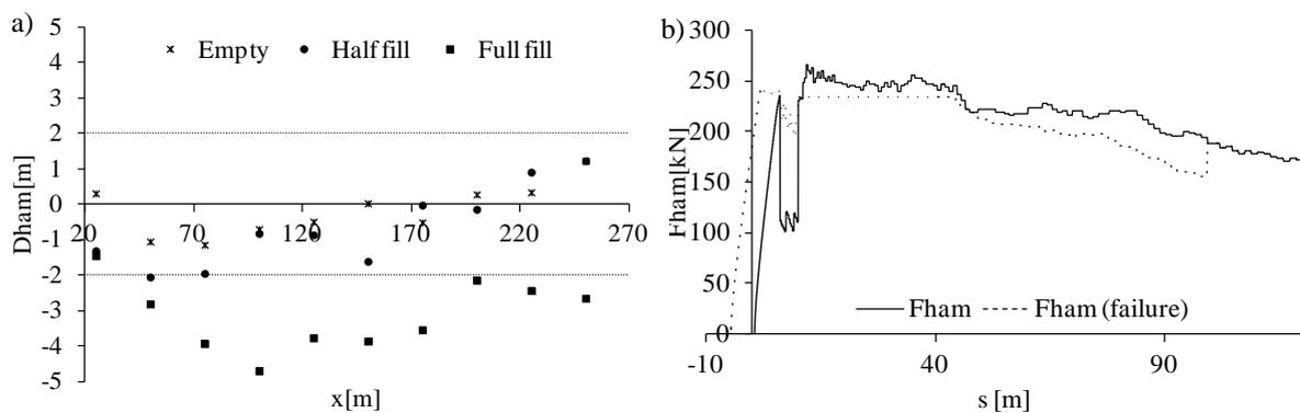
Fig. 8. a) Scattering of stopping points as the distance to the stopping point at which the state of failure and the impact on the accuracy of train have occurred ( $\pm 2$  is the stopping tolerance); b) mapping the braking force during the failure of a propulsion car ( $F_{ham\ failure}$ ) and the standard activity of braking during docking ( $F_{ham}$ )
