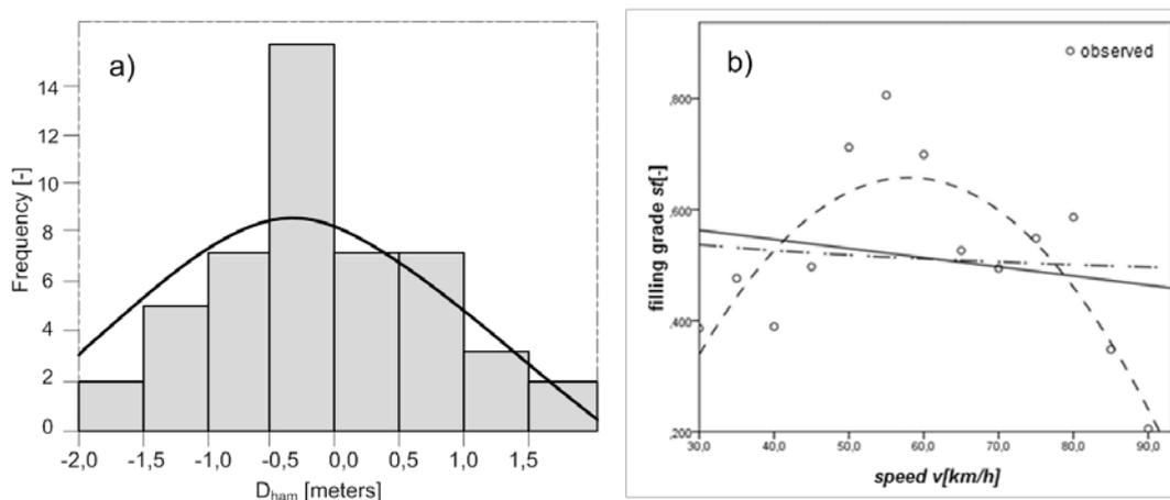
Fig. 10. a) A histogram of simulation outcomes of braking precision  $D_{ham}$  with a normal distribution curve; b) adjusting of the regression model for  $D_{ham}$  developed for the results of simulation (solid line—linear- regression function, the dotted line—logarithmic function, and intermittent line—the quadratic function)
