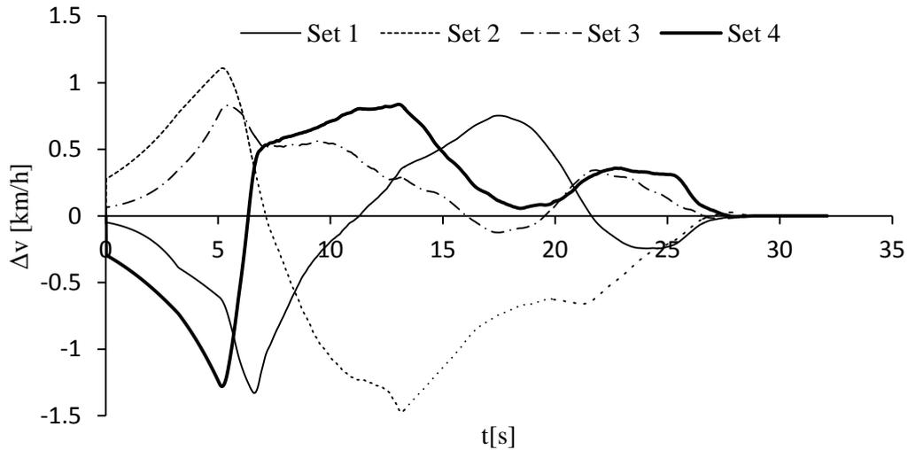
Fig. 6. The suppressed oscillatory course for adopted sets of terms of controller parameters; the degree of filling  $st=1,0$ ; speed of initiation of braking  $v_p=80$  km/h, and the complex route profile
