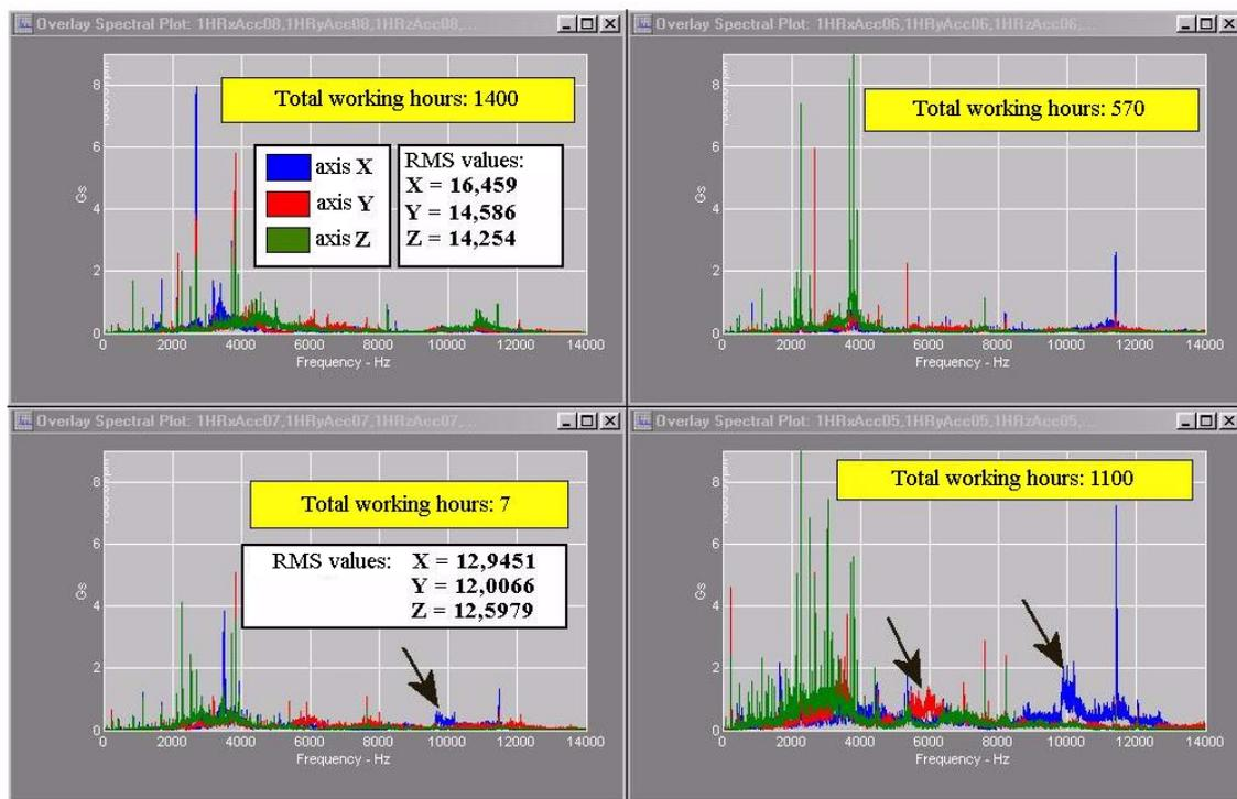
Fig. 4. Comparison of vibration spectra from main helicopter gearbox
