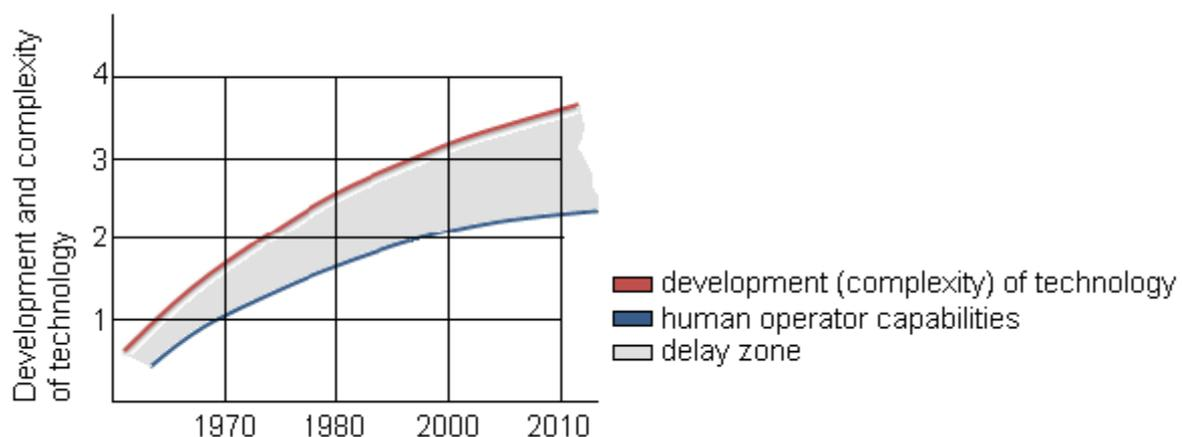
Fig. 3. The ratio of technology development (complexity) and the growth of human operator capabilities [6]
