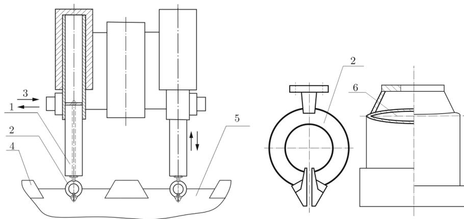
Fig. 2. Tamping unit schematic diagram
