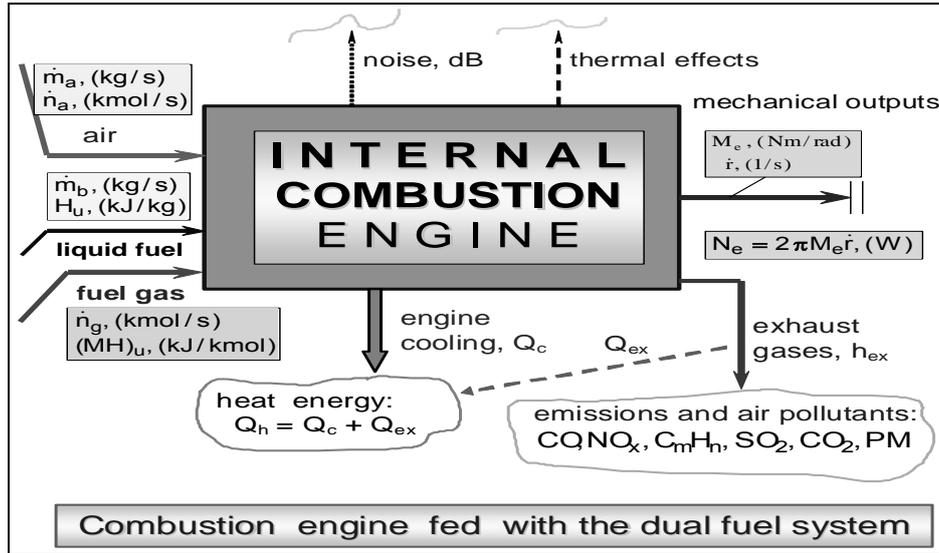
Fig. 2. Internal combustion engine with a dual fuel supply system
