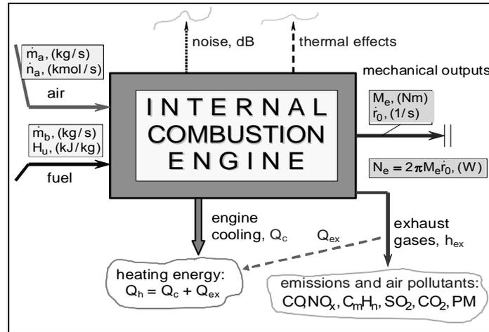
Fig. 1. Classic IC engine system and its parameters
