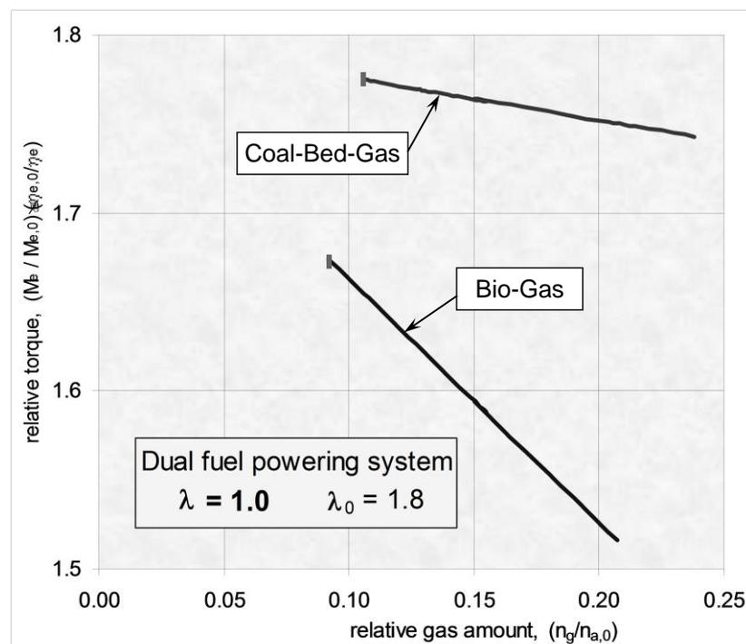
Fig. 6. Influence of gaseous fuels on the relative torque of the IC engine working at the full load state
