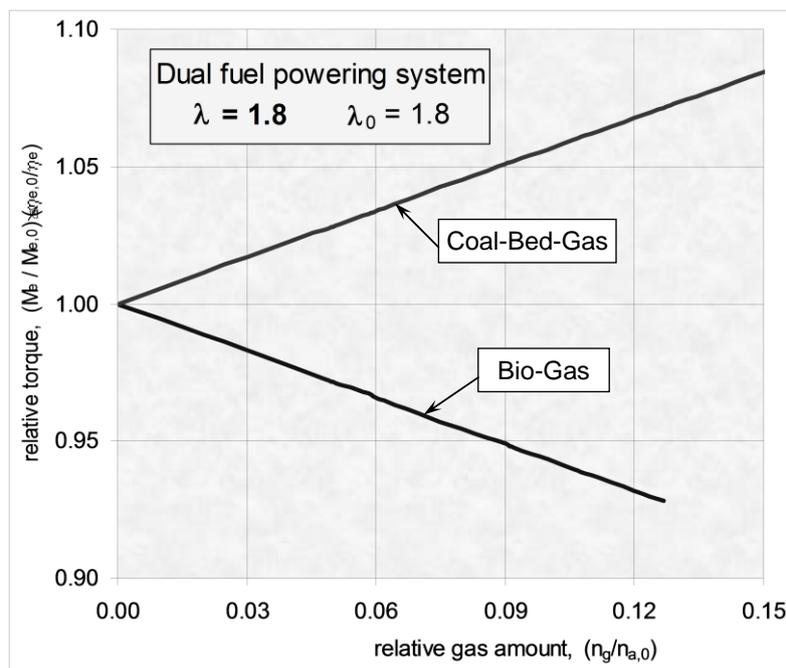
Fig. 5. Influence of gaseous fuels on the relative torque of the engine working at the reference state
