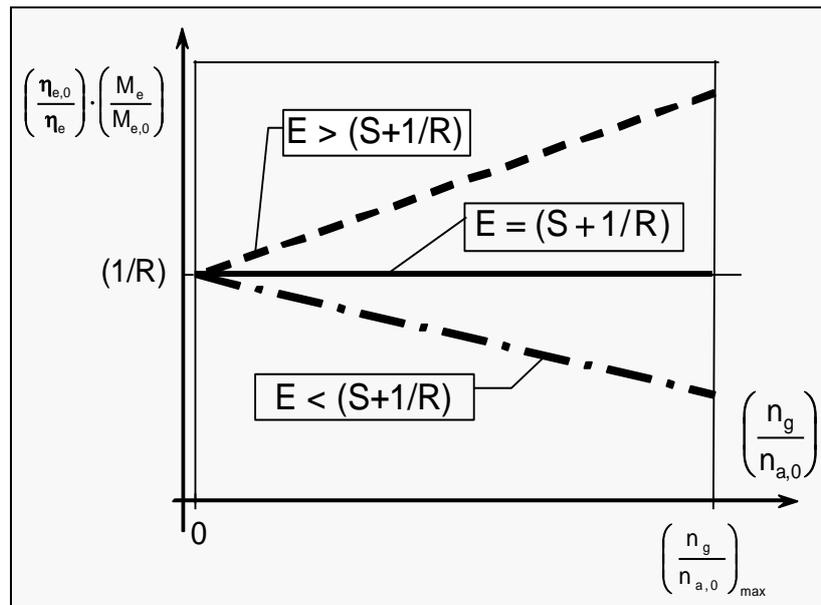
Fig. 4. Performance parameters of the engine working with the dual fuel system
