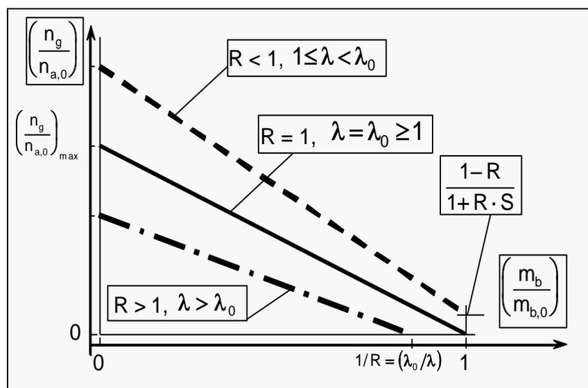
Fig. 3. Relative amount of gaseous fuel and liquid fuel in the engine cylinder
