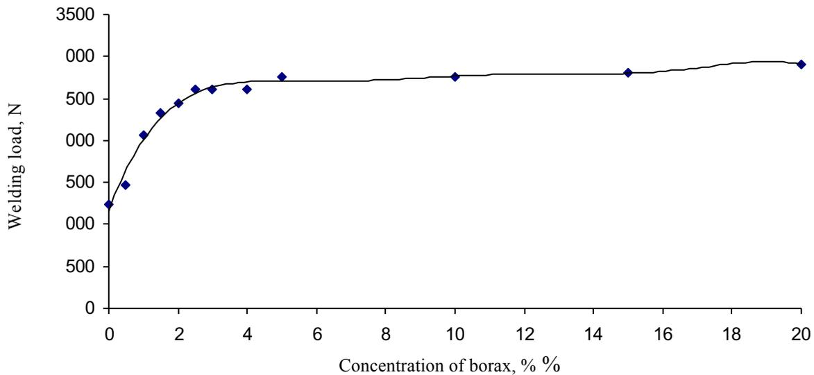
Fig. 2. Relation between welding load and borax concentration
