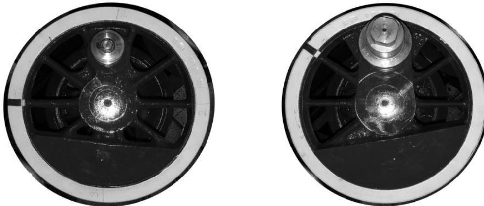
Fig. 2. Comparison of coupled wheel and driving wheel counterbalances, showing that the counterbalance must be shifted clockwise
