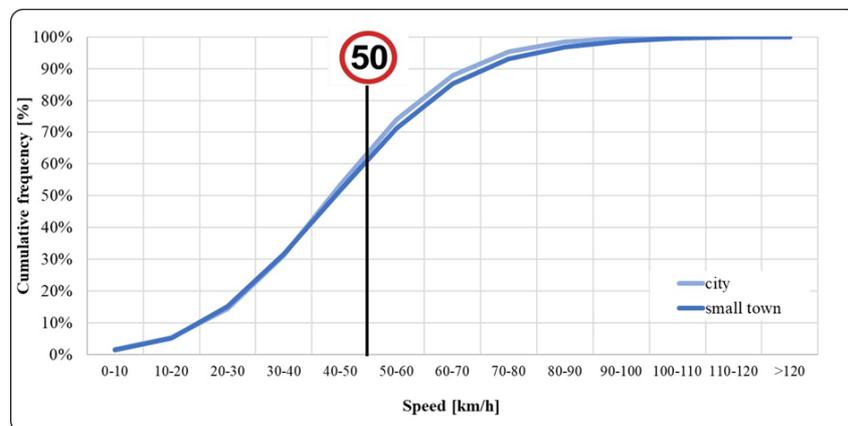
Fig. 7. Distribution of a speed of 10 m before a pedestrian crossing in cities and small towns – V limit = 50 km / h [12]
