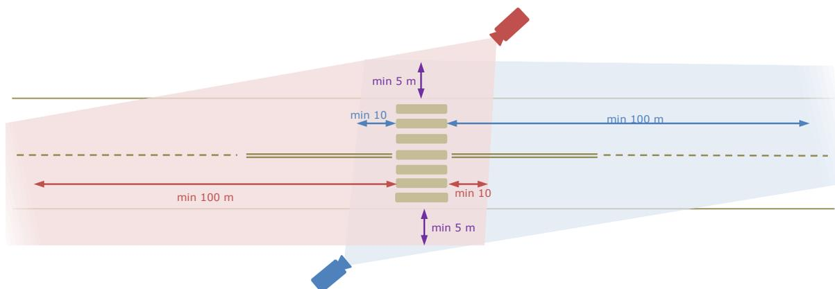
Fig. 5. Camera installation method - top view [12]
