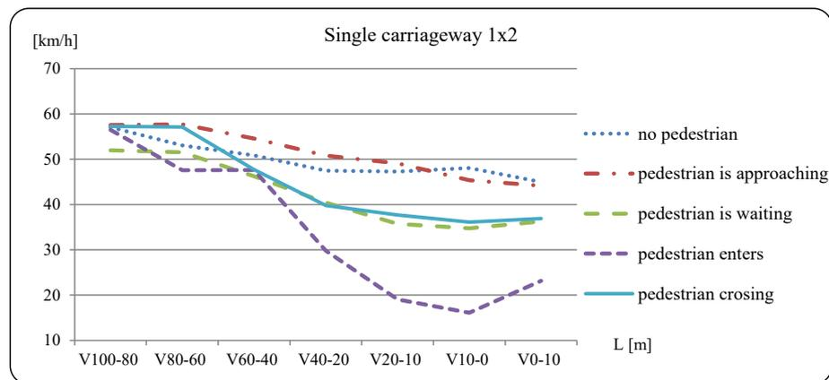
Fig. 11. Vehicle speed characteristics in the area of pedestrian crossings - permitted speed 50 km/h - average speed at 100 m before and up to 10 m after the pedestrian crossing [12]
