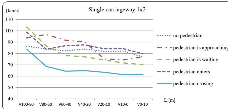
Fig. 10. Characteristics of vehicle speed in the area of pedestrian crossings - permitted speed 70 km/h - average speed at a distance up to 100 m before and up to 10 m after the pedestrian crossing [12]
