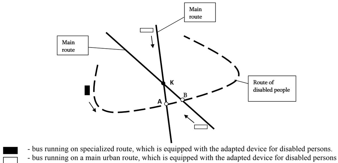
Fig. 3. Scheme of the intersection of specialized route with a main urban route (1<sup>st</sup> case) A and B – intersection points, K – destination
